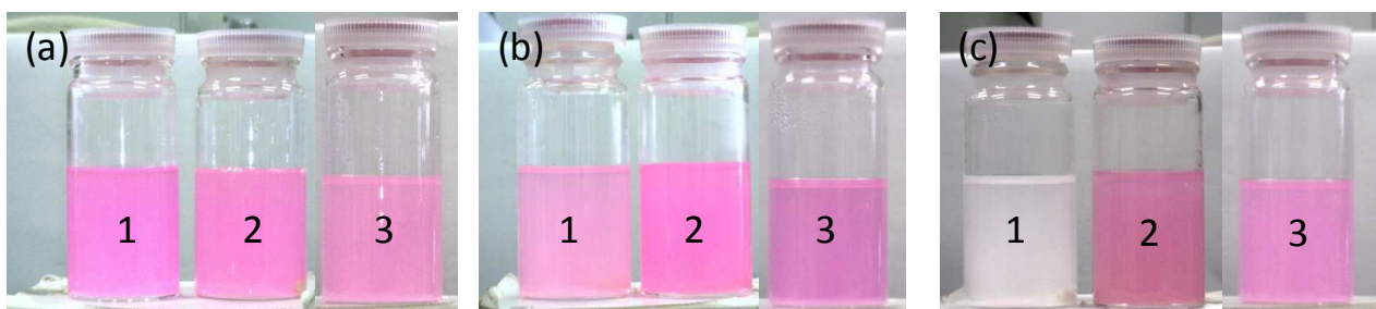
Figure 12. Investigation of influence of the monomer unit (aliphatic and aromatic carboxylic acids), (1) \text{TiO}_2 , (2) \text{TiO}_2 /phthalic acid (PA), (3) \text{TiO}_2 /methylsuccinic acid (MSA). UV irradiated (a) 0 min, (b) 60 min, (c) 120 min.
