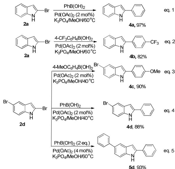
**Scheme 3.** The Suzuki coupling of **2a** and **2d** with arylboronic acids.
