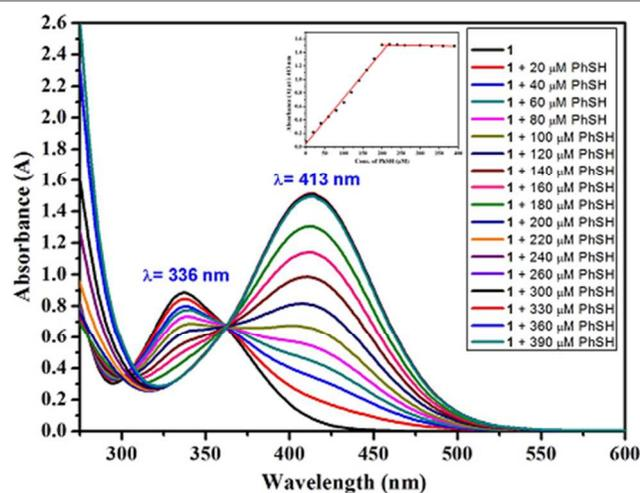
**Fig. 2** Effect of [PhSH] on the absorption spectra of **1** ( $\lambda = 336$  nm) was studied in PBS buffer (10mM, pH 7.4) with 25% acetonitrile as co-solvent. Significant red shift observed to  $\lambda = 413$  nm upon addition of PhSH (upto 2 equiv). This shift in wavelength ( $\Delta\lambda = 77$  nm) resulted into visual color change from colourless to bright yellow. Inset: Absorbance at 413 nm as a function of PhSH concentration indicates 1:2 ratio for probe **1** and PhSH.
