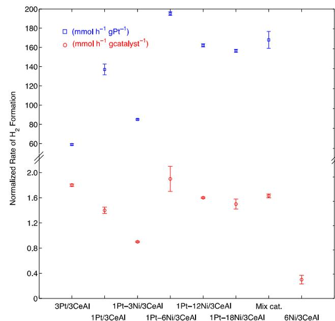
**Figure 6.** Rate of H<sub>2</sub> production from the APR of glycerol (240 °C, 40 bar, 1 wt% glycerol, 0.05 mL min<sup>-1</sup>, 250 mg catalyst; data are mean values over  $t = 5\text{--}20$  h), normalized to the mass of catalyst or Pt used. Error bars indicate one standard deviation; each data point is the average of  $\geq 2$  experiments. Mix cat. = mixture of separate Pt/3CeAl and Ni/3CeAl catalysts with a total of 1 wt% Pt and 6 wt% Ni.
