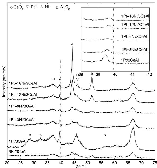
**Figure 2.** X-ray diffraction patterns of catalysts that had been reduced in flowing H<sub>2</sub> (50 vol.% in N<sub>2</sub>) at 800 °C for 60 min (heating rate 1.5 °C min<sup>-1</sup>). 1Pt/3CeAl was reduced at 500 °C. Inset shows the Pt (111) peak region.
