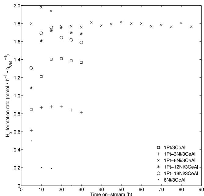
**Figure 7.** Variation of  $\text{H}_2$  formation rate with time on-stream in the APR of glycerol (240 °C, 40 bar, 1 wt% glycerol, 0.05 mL min<sup>-1</sup>, 250 mg catalyst). Each value is the average of  $\geq 2$  experiments. The best catalyst, 1Pt-6Ni/3CeAl, was tested in an extended run.
