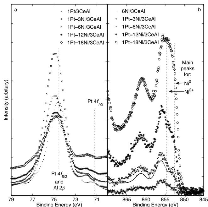
**Figure 3** The Pt 4f and Al 2p region of the X-ray photoelectron spectra of xPt-yNi/3CeAl catalysts that had been reduced in flowing H<sub>2</sub> (50 vol.% in N<sub>2</sub>) at 800 °C for 60 min (heating rate 1.5 °C min<sup>-1</sup>). 1Pt/3CeAl was reduced at 500 °C.
