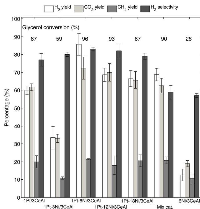
**Figure 4** Effect of adding Ni to Pt/3CeAl catalysts on yields, selectivity and glycerol conversions in the aqueous phase reforming of glycerol (240 °C, 40 bar, 1 wt% glycerol, 0.05 mL min<sup>-1</sup>, 250 mg catalyst; data are mean values over  $t = 5$ –20 h). Error bars indicate one standard deviation; each bar is the average of  $\geq 2$  experiments. Mix cat. = mixture of separate Pt/3CeAl and Ni/3CeAl catalysts with a total of 1 wt% Pt and 6 wt% Ni.
