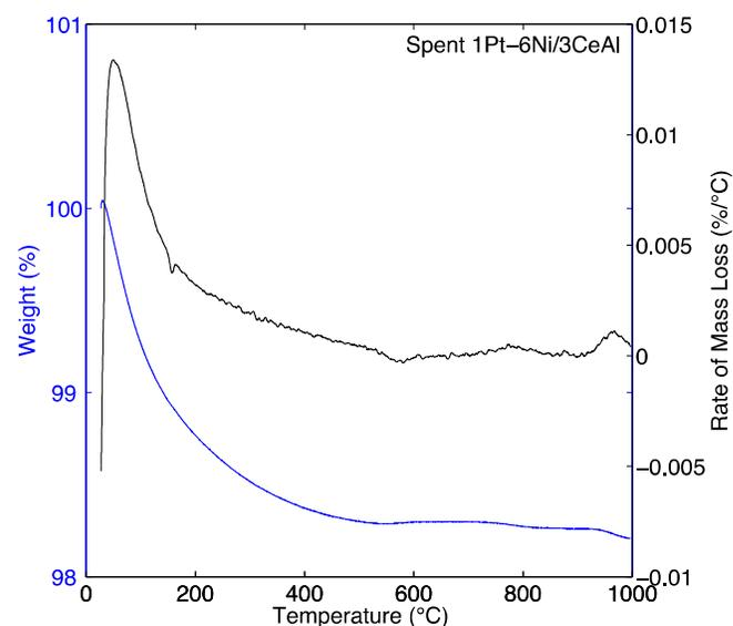
**Figure 9.** Thermogravimetric analysis of fresh (reduced: 50 vol%  $\text{H}_2$  in  $\text{N}_2$ , 800 °C, 60 min) and spent (after reaction: 240 °C, 40 bar, 1 wt% glycerol, 0.05 mL min<sup>-1</sup>, 85 h) 1Pt-6Ni/3CeAl. Samples were heated at 10 °C min<sup>-1</sup> in instrument air (40 vol% in  $\text{N}_2$ ).
