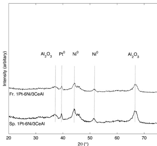
**Figure 8.** XRD patterns of 1Pt-6Ni/3CeAl catalyst freshly reduced in flowing  $\text{H}_2$  (50 vol% in  $\text{N}_2$ ) at 800 °C for 60 min, and spent after 30 h on-stream (240 °C, 40 bar, 1 wt% glycerol, 0.05 mL min<sup>-1</sup>, 250 mg catalyst).
