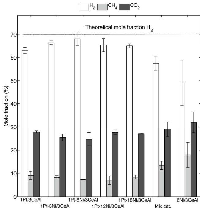
**Figure 5.** Effect of Ni addition to Pt/3CeAl catalysts on the distribution of gaseous products from the aqueous phase reforming of glycerol (240 °C, 40 bar, 1 wt% glycerol, 0.05 mL min<sup>-1</sup>, 250 mg catalyst; data are mean values over  $t = 5\text{--}20$  h). Error bars indicate one standard deviation; each bar is the average of  $\geq 2$  experiments. Mix cat. = mixture of separate Pt/3CeAl and Ni/3CeAl catalysts with a total of 1 wt% Pt and 6 wt% Ni.
