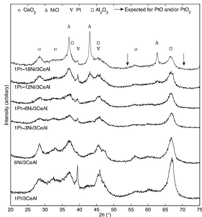
**Figure 1.** X-ray diffraction (XRD) patterns of xPt-yNi/3CeAl catalysts that had been calcined at 600 °C for 6 h under air (heating rate 1.5 °C/min).
