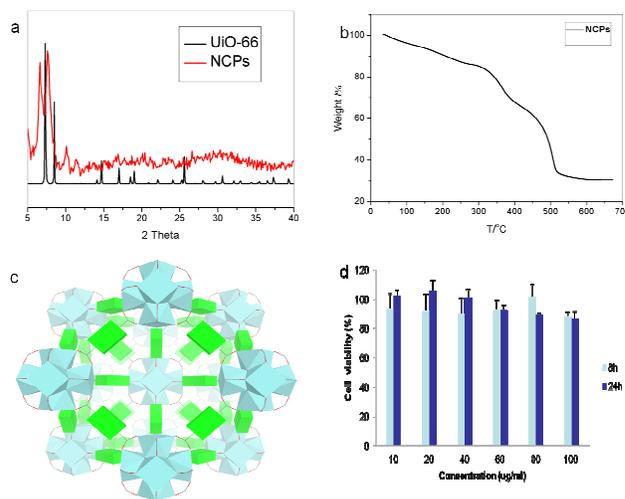
**Fig. 2** (a) PXRD of as synthesized NCPs (red) and UiO-66 (black). (b) TGA. (c) Simulated structure of NCPs, the green parts represent the ligand, colors of atoms O (red), Zr (light blue); MTT (d) of Hela cells after NCPs endocytosis.
