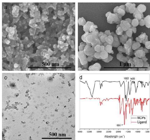
**Fig. 1** SEM (a, b) and TEM (c) of the NCPs. FT-IR Spectroscopy (d) of the ligand (red) and the particles (black).
