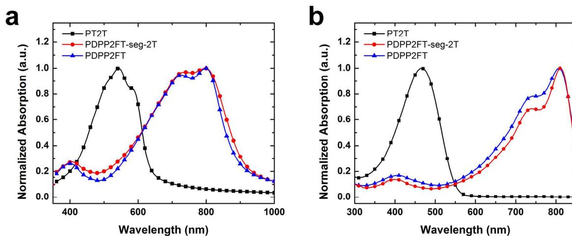
**Figure 4.** Absorption spectra of the three polymers synthesized in this work. (a) Thin films of the pure polymers spin cast from 4:1 chloroform:ODCB and (b) the pure polymers in chloroform at a concentration of  $1 \times 10^{-5}$  M.
