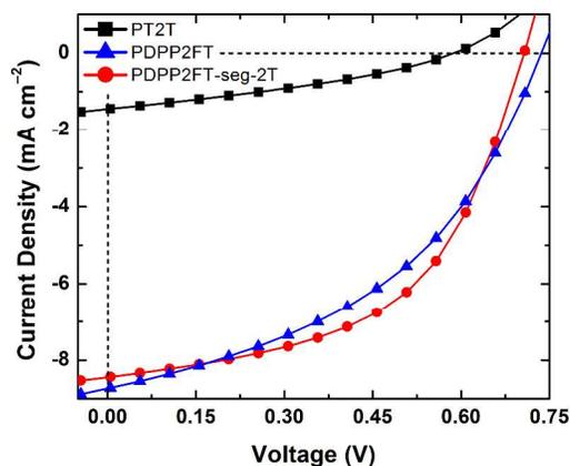
**Figure 6.** Photovoltaic characteristics of representative samples of polymer-fullerene blends. All active layers comprised 1:2 polymer:PC<sub>61</sub>BM.
