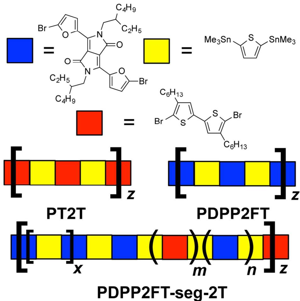
Random segmentation of unlike conjugated monomers within a low-bandgap polymer produces increased mechanical compliance without sacrificing photovoltaic performance.
