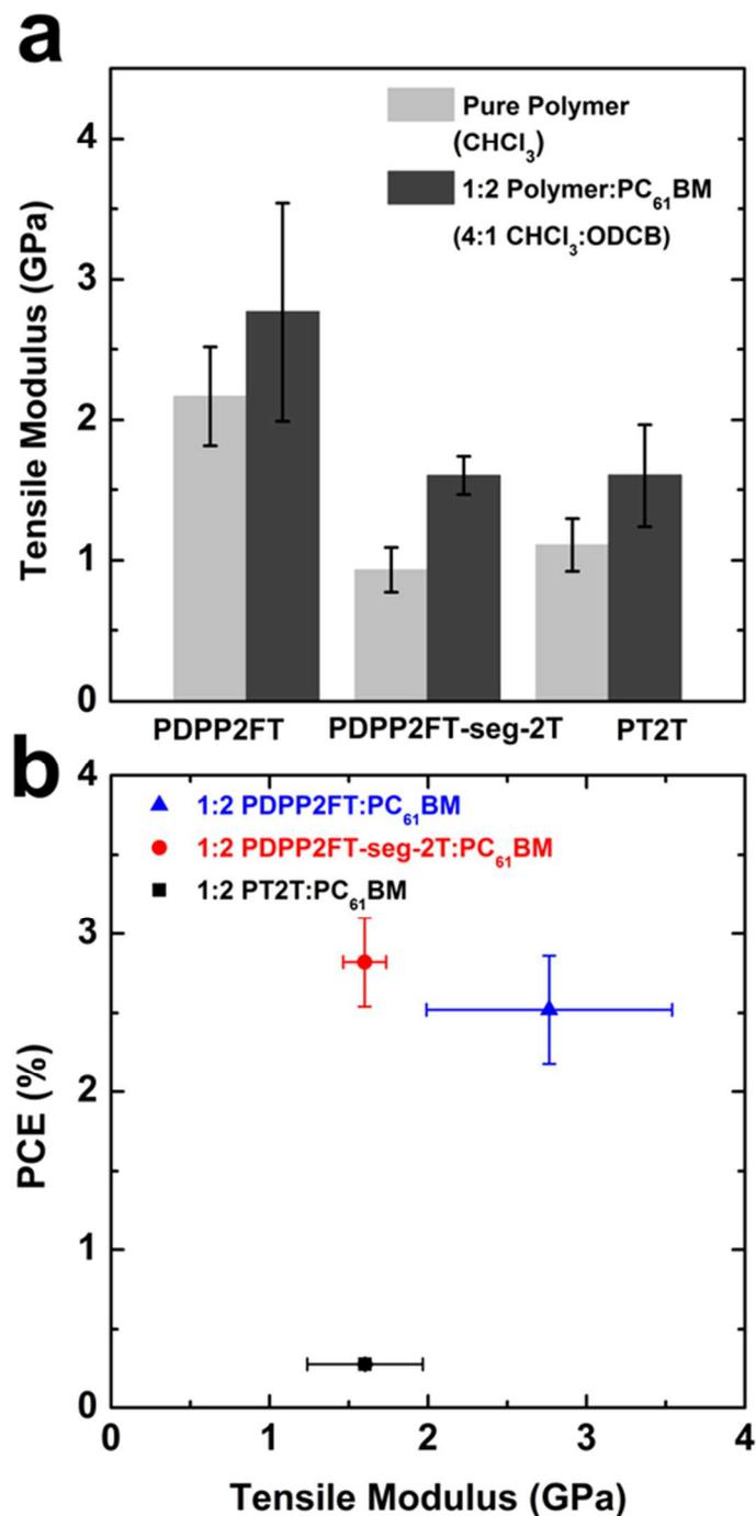
**Figure 8.** Mechanical properties of pure polymers and polymer:fullerene composites. (a) Comparison between the tensile moduli of pure polymer films spin-coated from chloroform and the films comprising 1:2 polymer:PC<sub>61</sub>BM blends spin-coated from 4:1 chloroform:ODCB. (b) Plot of power conversion efficiency of the polymers in a 1:2 blend with PC<sub>61</sub>BM spin-coated from 4:1 chloroform:ODCB. The architecture of the devices was
