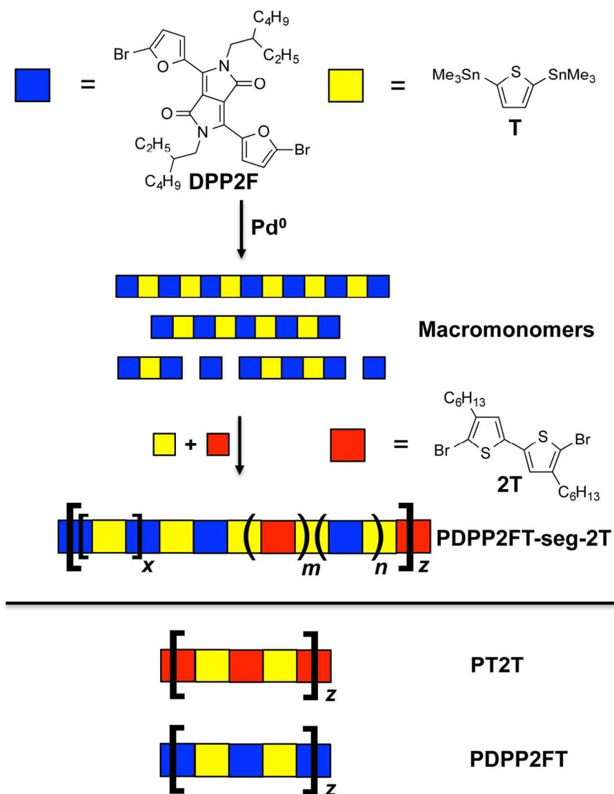
**Figure 2.** Summary of the synthetic strategy used to generate segmented copolymers. Two monomers, the dibromide (DPP2F) and the distannane (T), are reacted in the presence of  $\text{Pd}^0$ . Shortly after initialization of the reaction (when “macromonomers” began to form), additional T and dibrominated bithiophene (2T) were added to the reaction mixture to form the segmented polymer, PDPP2FT-seg-2T. Separately, the homopolymers PT2T and PDPP2FT were also prepared.
