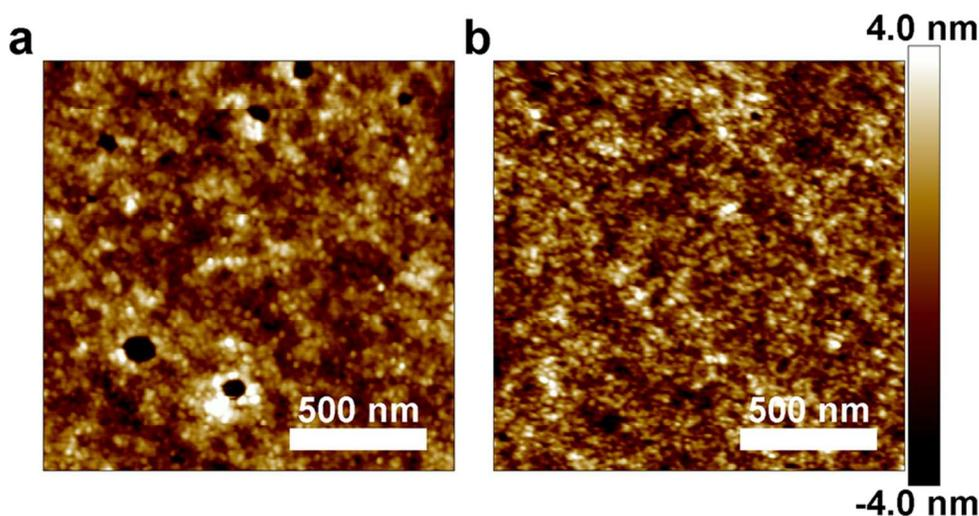
**Figure 7.** Height images from atomic force micrographs of unannealed polymer thin films. (a) PDPP2FT and (b) PDPP2FT-seg-2T.
