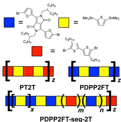
**Graphical abstract.** Random segmentation of unlike conjugated monomers within a low-bandgap polymer produces increased mechanical compliance without sacrificing photovoltaic performance.
