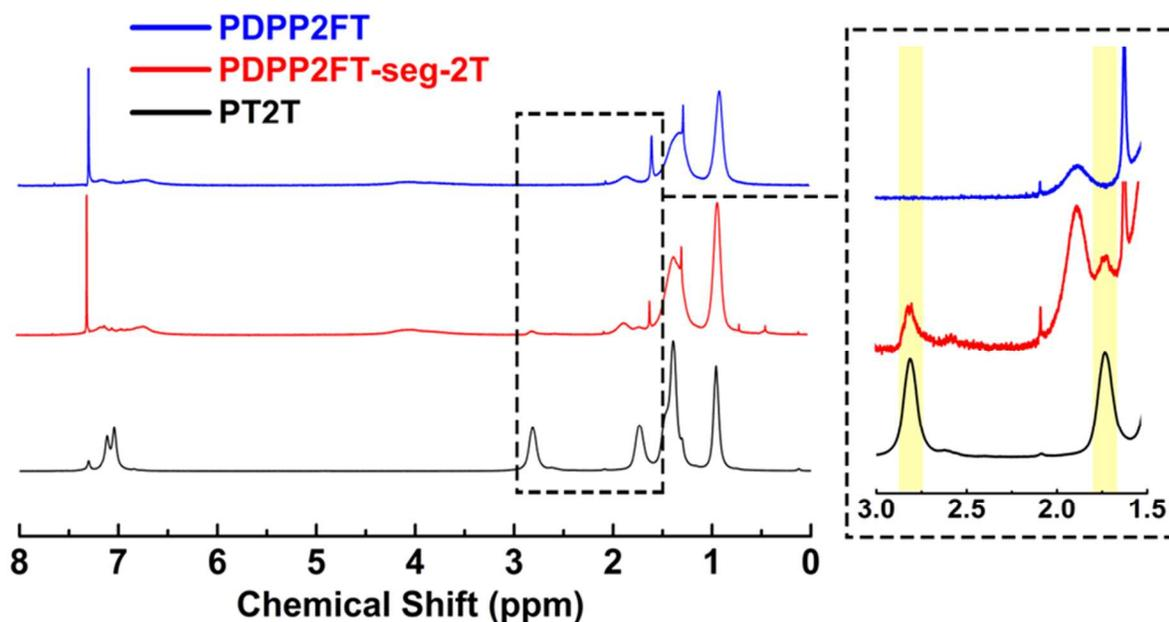
**Figure 3.**  $^1\text{H}$  NMR spectra of PDPP2FT, PDPP2FT-seg-2T, and PT2T. Peaks associated with the bithiophene are highlighted in the inset at  $\delta = 2.88\text{-}2.38$  ppm and  $1.74\text{-}1.63$  ppm.
