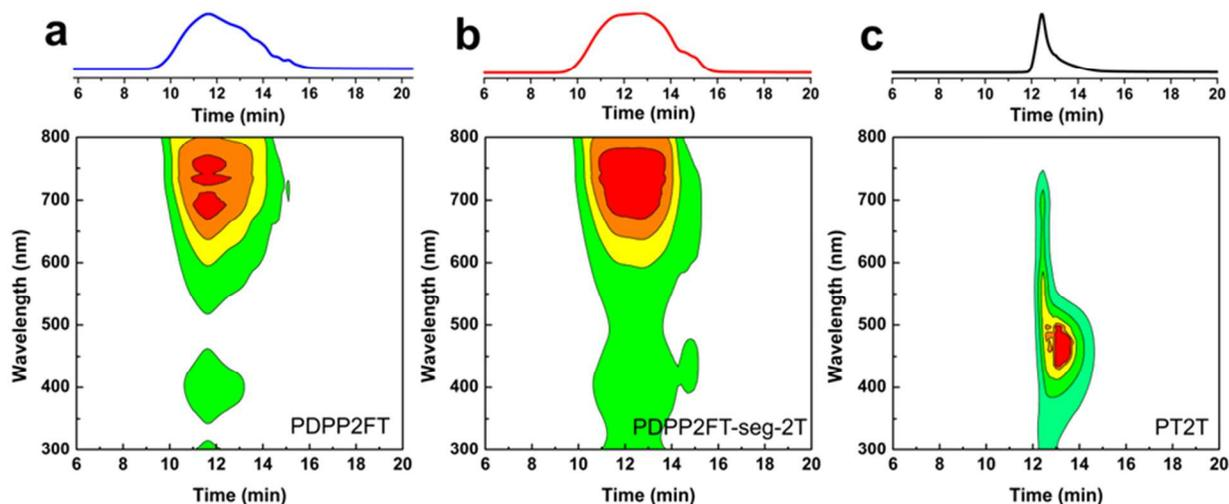
**Figure 5.** GPC traces and contour plots for (a) PDPP2FT, (b) PDPP2FT-seg-2T, and (c) PT2T based on a UV detector.
