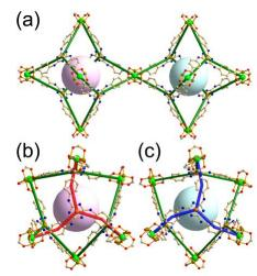
Figure 8. A 3-D network of **tbo** topology based on the 3-c node of  $C_3$  point symmetry. (a) The alternating tetrahedral MOPs in the network of tbo topology. (b) A view showing the  $C_3$  point symmetry ligand of a right-handed  $C_3$  rotational symmetry in MOP-A. (c) A view showing the  $C_3$  point symmetry ligand of a left-handed  $C_3$  rotational symmetry in MOP-B.
