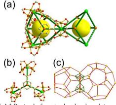
Figure 15. A 3-D network of moo topology based on a heterocubic MOP. (a) The heterocubic MOPs are corner-shared, where the orange spheres represent 3-c BTC ligands and the green spheres represent corner-shared 6-c SBUs. (b) The BTC ligand in the heterocubic MOP is linked to three 55 6-c SBUs. (c) The corner-shared heterocubic MOPs generate a net of mtn underlying topology based on a heterocubic MOP as a TBU.
