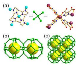
Figure 45. A 4-c zeolitic net of sod topology. (a) The meim or the Himdc ligand serves as a 2-c node and the [Zn(Nmeim)<sub>4</sub>] unit or the In(III) center serves as a tetrahedral 4-c node. (b) The two truncated octahedral MOPs (sod cages) are interlinked via face-sharing of the four square-nodes of 80 the sod cages in a square arrangement (4R linkage). (c) The net contains the same *sod* cage at the body-center of the face-shared *sod* cages.
