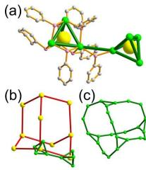
Figure 2. A 3-D network of **dia-a** topology based on the tetrahedral MOP <sup>65</sup> [Cd<sub>4</sub>(SPh)<sub>6</sub>]. (a) The tetrahedral MOP serves as a 4-c SBU through four outer SPh bridging ligands. (b) The adamantine cage of **dia** underlying topology based on the tetrahedral MOP. (c) The adamantinoid supercage of truncated tetrahedral geometry.
