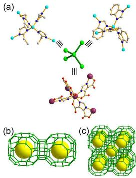
Figure 47. A 4-c zeolitic net of rho topology. (a) The eim or the phim or the Himdc ligand serves as a 2-c node and the  $[Zn(N_{eim})_4]$  or the  $[Zn(N_{phim})_4]$  or the  $[In((N\sim O)_{Himde})_4]$  unit serves as a tetrahedral 4-c node. (b) The two lta cages are interconnected via octupule corner linkage between the eight 4-c nodes of the *lta* cages in an octagonal arrangement (d8R linkage). (c) The net contains the same lta cage at the body-center.
