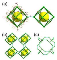
60 Figure 38. A 3,5-c network of jjp topology based on a partially corner-linked rhombic dodecahedral MOP. (a) Rhombic dodecahedral MOP with orange vertices representing 3-c organic nodes and green vertices representing 4-c copper ions is interlinked via the 4-c corners of the MOP. (b) The MOP as a 6-c SBU is connected via a 2-c nitrate anion to a net of
