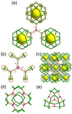
Figure 30. A 3,3,4-c network of **ntt** topology based on a cuboctahedral 55 MOP. (a) The three cuboctahedral MOPs are linked by the 3-c organic node. (b) The ligand consisting of two different kinds of four 3-c nodes is connected to six 4-c inorganic nodes. (c) Scheme of a 3,24-c rht underlying topology. (d) and (e) The two kinds of supercages derived from an octahedron and a tetrahedron, respectively.
