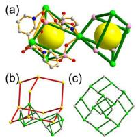
Figure 13. A 3-D network of spn topology based on a heterocubic MOP. (a) The partially corner-shared heterocubic MOPs, where the pink spheres 20 represent 3-c 3-ppp ligands and the green spheres represent corner-shared 6-c cadmium ions. (b) A net of the corner-shared heterocubic MOPs of dia underlying topology. (c) The supercage of a 4<sup>6</sup>.12<sup>4</sup> face symbol derived from adamantinoid geometry.
