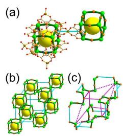
Figure 19. A 3,3,3-c network of rqz topology based on a partially edgecenter-linked cubic MOP. (a) The cubic MOPs are linked via the edgecenters of the cubic MOP. (b) The network of pcu underlying topology showing the primitive cubic close packing arrangement of the cubic 5 MOPs. (c) The supercage of an 186 face symbol. The pink dotted lines show the cubic geometry of the supercage.
