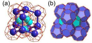
45 Figure 6. (a) Ball-and-stick and (b) tile-and-net models of a net of mtn topology with dodecahedral cages (blue) in dia underlying topology and with the four mtn cages (cyan) in adamantinoid supercage.
