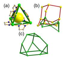
Figure 3. A 3-D network of **dia-e** topology. (a) The tetrahedral MOP  $[Pr_4(im)_6]$ . (b) The 6-c **crs** net based on the tetrahedral MOP as a corner-shared SBU. (c) The truncated tetrahedral supercage.
