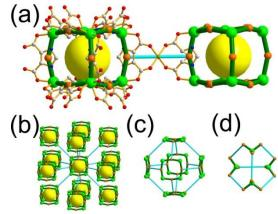
45 Figure 18. A network of xaa topology based on a cubic MOP. (a) The cubic MOPs are interconnected via the edge-center through the ditopic linker [Zn(COO)<sub>4</sub>]. (b) The network of fcu underlying topology showing the cubic close packing arrangement of the cubic MOPs. The two different kinds of supercages of (c) a polyhedron of an 8<sup>6</sup>.9<sup>8</sup> face symbol 50 and (d) a polyhedron of a 9<sup>4</sup> face symbol.
