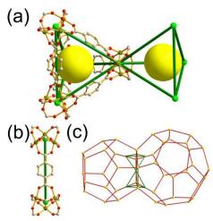
40 Figure 5. A 3-D network of mtn-e topology based on a tetrahedral MOP. (a) Four 6-c trinuclear [M<sub>3</sub>O(COO)<sub>6</sub>] SBUs are connected by six BDC ligands to a corner-shared tetrahedral MOP. (b) The linkage between the [M<sub>3</sub>O(COO)<sub>6</sub>] SBUs. (c) The tetrahedral MOPs are corner-shared to a net of mtn underlying topology.
