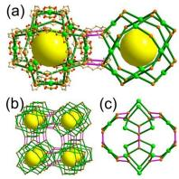
Figure 29. A 3-D network of zhc topology based on a cuboctahedral 25 MOP. (a) The cuboctahedral MOPs are quadruply linked via the edgecenters of the cuboctahedral MOP. (b) Scheme of the net of pcu
