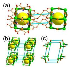
Figure 20. A 3,3-c network of tfg/P topology based on a doubly edgecenter-linked cubic MOP. (a) The cubic MOPs are doubly linked via the edge-centers of the cubic MOP. (b) The network of pcu underlying topology showing the primitive cubic close packing arrangement of the 20 cubic MOPs. (c) A supercage of a 126 face symbol.
