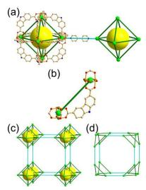
50 Figure 22. A 3-D network of cab topology based on an octahedral MOP. (a) The octahedral MOP assembled from 12 cdc ligands as a 90°-bent 2-c linker and six [Cu<sub>2</sub>(COO)<sub>4</sub>] SBUs as a planar 4-c corner is corner-linked via a linear 2-c bipy linker. (b) A 2-c 90°-bent linker. (c) Scheme of pcua topology with the octahedral MOP as a TBU. (d) The truncated cubic 55 supercage of a 38.86 face symbol.
