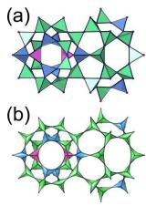
Figure 16. A comparison between the nets of (a) **mtn-e** topology and (b) **moo** topology.
