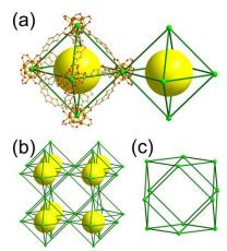
15 Figure 23. A 3-D network of reo topology based on an octahedral MOP. (a) An octahedral MOP based on six [Zr<sub>6</sub>O<sub>6</sub>(OH)<sub>2</sub>(COO)<sub>8</sub>] clusters interlinked via 12 2-c dttdc linkers. (b) Scheme of pcu-e topology with the corner-shared octahedral MOP. (c) The cuboctahedral supercage of a 38.46 face symbol.
