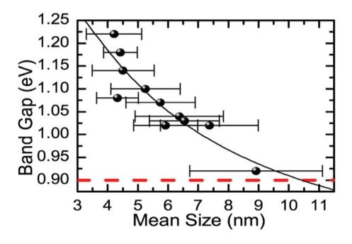
Figure 15. Relationship between the energy of the band gap and the mean size (diameter) for SnSe nanocrystals produced by Baumgardner *et al.* using thermolysis.<sup>67</sup> Reprinted with permission from Baumgardner *et al. J. Am. Chem. Soc.* 2010, 132, 9519-9521. Copyright 2010 American Chemical Society.
