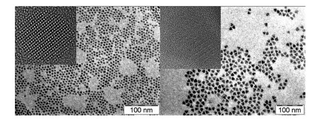
Figure 7. TEM and HRTEM (insets) of spherical and triangular SnS nanocrystals produced by Eychmüller and co-workers via hot injection-thermolysis of precursors.<sup>30</sup> Reprinted with permission from Hickey et al. J. Am. Chem. Soc. 2008, 130, 14978-14980. Copyright 2008 American Chemical Society.
