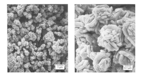
**Figure 12.** SnSe produced by Bahr *et al.* from a cyclic single source precursor of the type (Ph<sub>2</sub>SeSn)<sub>3</sub>.<sup>53</sup> Reprinted with permission from Bahr *et al. Chem. Mater.* 1992, **4**, 383-388. Copyright 1992 American Chemical Society.
