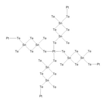
Figure 22. Platinum tin telluride structure deduced by Riley and Tolbert from EXAFS data.<sup>107</sup>
