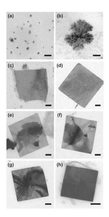
Figure 14. TEM study of growth mechanism of SnSe nanosheets by Vaughan II *et al.*<sup>62</sup> Images a) and b) represent nucleation, c) and d) lateral growth from nanoparticle attachment whilst images e) to h) represent layer by layer vertical growth. All scale bars 100 nm. Reprinted with permission from Vaughan II *et al. ACS Nano* 2011, 5, 8852-8860. Copyright 2011 American Chemical Society.
