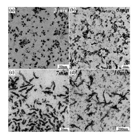
Figure 19. Temporal study of the *oriented attachment* mechanism of SnSe nanowire growth by Ning *et al.*<sup>76</sup>
