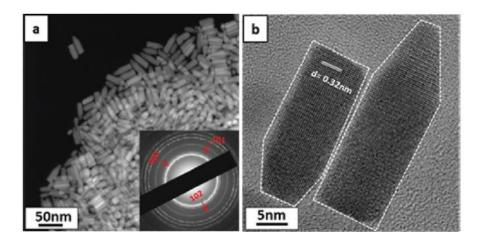
**Figure 20.** DF-STEM and HR-TEM images of bullet-shaped CZTS nanorods produced by Ryan and coworkers.<sup>84</sup> (a) DF-STEM image of nanorods inset: SAED pattern revealing wurtzite phase. (b) HR-TEM image of two nanorods revealing elongation in the [002] direction. Reprinted with permission from Singh *et al. J. Am.*
