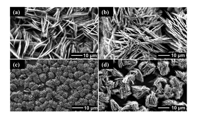
Figure 6. SEM images of SnS films deposited on glass substrates from [Sn(C<sub>4</sub>H<sub>9</sub>)<sub>2</sub>(S<sub>2</sub>CN(C<sub>4</sub>H<sub>9</sub>)<sub>2</sub>)<sub>2</sub>]. (a) 450 °C,
