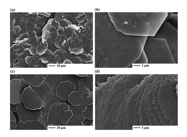
**Figure 11.** SEM images of SnSe thin films produced by Parkin and co-workers by APCVD from two different ratios of tin(IV) chloride to diethyl selenide. a) & b)  $SnCl_4:Et_2Se = 1:1. c$ ) & d)  $SnCl_4:Et_2Se = 10:1.^{51}$  Reprinted from Boscher *et al. Thin Solid Films* 2008, **516**, 4750-4757. Copyright 2008, with permission from Elsevier.
