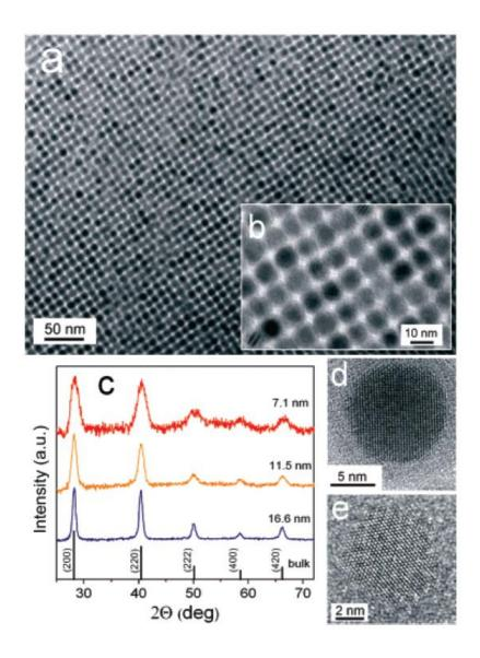
Figure 18. (a), (b) TEM images of SnTe NCs capped with oleic acid. (c) Powder XRD patterns of SnTe NCs with various sizes. (d), (e) HRTEM of SnTe NCs viewed along [001] and [111] zone axes.<sup>75</sup> Reprinted with permission from Kovalenko *et al. J. Am. Chem. Soc.* 2007, **129**, 11354-11355. Copyright 2007 American Chemical Society.
