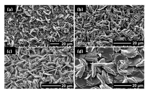
Figure 5. SEM images of SnS films deposited f on glass substrates from [Sn(C<sub>4</sub>H<sub>9</sub>)<sub>2</sub>(S<sub>2</sub>CN(C<sub>2</sub>H<sub>5</sub>)<sub>2</sub>)<sub>2</sub>] at (a) 450 °C, (b) 500 °C, and from [Sn(C<sub>4</sub>H<sub>9</sub>)<sub>2</sub>(S<sub>2</sub>CN(CH<sub>3</sub>)(C<sub>4</sub>H<sub>9</sub>))<sub>2</sub>] (c) 450 °C and (d) 500 °C.<sup>27</sup> Reprinted with permission from Ramasamy *et al. Chem. Mater.* 2013, 25, 266-276. Published 2013 American Chemical
