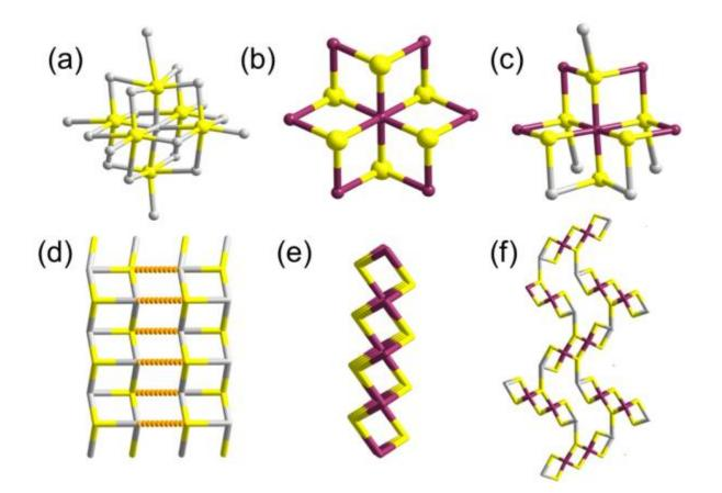
Figure 1. Local Sn environments in (a) SnS, (b) SnS<sub>2</sub> and (c) Sn<sub>2</sub>S<sub>3</sub>; and Sn...S connectivity in (d) SnS, (e) SnS<sub>2</sub> and (f) Sn<sub>2</sub>S<sub>3</sub>. (Sn(II)-grey, Sn(IV)-violet, S-yellow). Reprinted with permission from Ramasamy *et al. Chem. Mater.* 2013, 25, 266-276. Published 2013 American Chemical Society.
