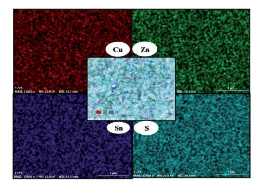
**Figure 21.** EDX elemental mapping of CZTS thin films produced by O'Brien and co-workers by using AACVD with a mix of three discrete molecular precursors.<sup>94</sup> Reproduced from Ref. 94 with permission from The Royal Society of Chemistry.
