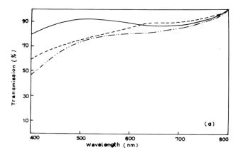
Figure 2. Visible transmission spectrum of SnS films produced by Ray *et al.* using dip deposition.<sup>6</sup> Reprinted from Ray *et al. Thin Solid Films*, 1999, **350**, 72-78. Copyright 1999 with permission from Elsevier.
