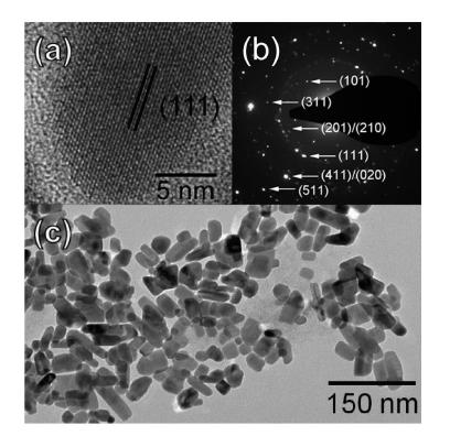
Figure 16. Imaging of SnSe nanocrystals produced by the method of Franzman *et al.* for use in solar cells. a) HRTEM of a single nanocrystal, b) SAED pattern with indexing of SnS crystal planes and c) TEM of SnSe nanocrystal ensemble.<sup>68</sup> Reprinted with permission from Franzman *et al. J. Am. Chem. Soc.* 2010, 132, 4060-4061. Copyright 2010 American Chemical Society.
