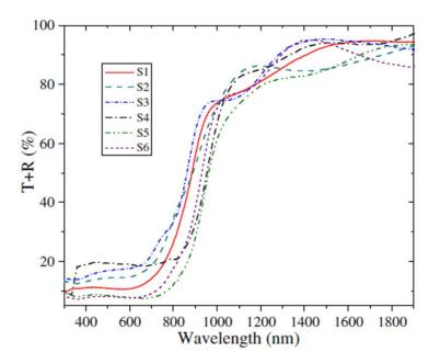
Figure 3: Combined transmittance-reflectance curves for SnS films produced by Gao and co-workers by chemical bath deposition with band gaps in the range 1.0 - 1.3 eV.<sup>12</sup> Reprinted from Gao *et al. Thin Solid Films*, 2012, **520**, 3523-3527. Copyright 2012 with permission from Elsevier.
