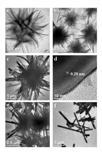
**Figure 8.** TEM images of the nanocrystalline products obtained at various reaction stages for the ratio of  $C_2H_5OCS_2K/SnCl_2 = 2.4$ : (a) 12 h, (b, c) 24 h, (d) HRTEM image of an individual SnS nanobelt, (e) 36 h, (f) 48
