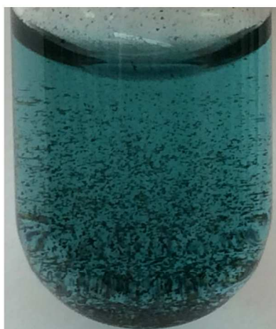
Figure 5. Visual observation of the disproportionation of [\text{CuBr}]_0/[\text{Me}_6\text{-TREN}]_0 = 1/1 at (a) 0 °C, and (b) 25 °C at different time intervals after stirring of the solution (for 5 min) was stopped. Conditions: \text{H}_2\text{O} = 1.8 \text{ mL} , [\text{CuBr}] = 15.2 \text{ mM} , [\text{CuBr}]/[\text{Me}_6\text{-TREN}] = 1/1 .
