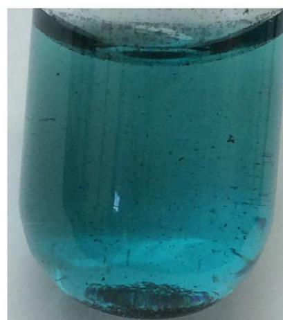
Figure 5. Visual observation of the disproportionation of [\text{CuBr}]_0/[\text{Me}_6\text{-TREN}]_0 = 1/1 at (a) 0 °C, and (b) 25 °C at different time intervals after stirring of the solution (for 5 min) was stopped. Conditions: \text{H}_2\text{O} = 1.8 \text{ mL} , [\text{CuBr}] = 15.2 \text{ mM} , [\text{CuBr}]/[\text{Me}_6\text{-TREN}] = 1/1 .
