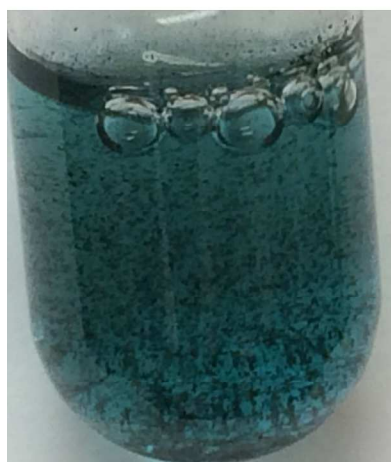
Figure 5. Visual observation of the disproportionation of [\text{CuBr}]_0/[\text{Me}_6\text{-TREN}]_0 = 1/1 at (a) 0 °C, and (b) 25 °C at different time intervals after stirring of the solution (for 5 min) was stopped. Conditions: \text{H}_2\text{O} = 1.8 \text{ mL} , [\text{CuBr}] = 15.2 \text{ mM} , [\text{CuBr}]/[\text{Me}_6\text{-TREN}] = 1/1 .
