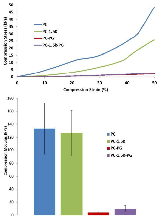
**Figure 5.** Mechanical properties of the PC hydrogel series using the unconfined compression test.
