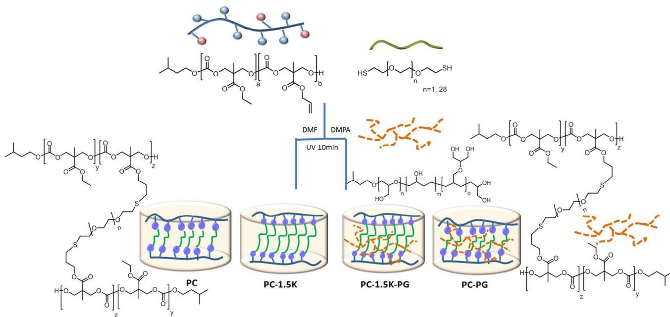
**Figure 1.** Synthesis of polycarbonate gels with short (PC, PC-PG) or long dithiol crosslinker (PC-1.5K, PC-1.5K-PG) in the presence (PC-PG, PC-1.5K-PG) or absence of polyglycidol (PC, PC-1.5K).
