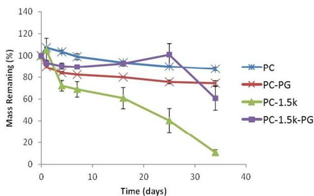
**Figure 4.** Degradation profiles of hydrogels in PBS at 37 °C
