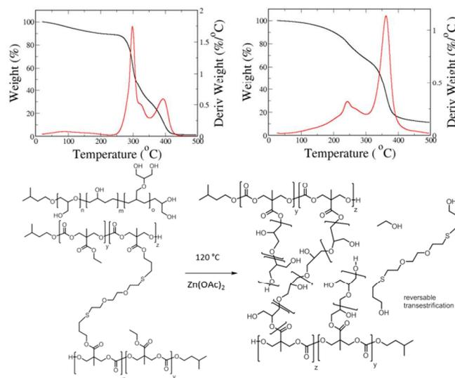
**Figure 2.** Thermogravimetric analysis of polycarbonate-polyglycidol hydrogel before (left) and after zinc acetate catalyzed transesterification (right).
