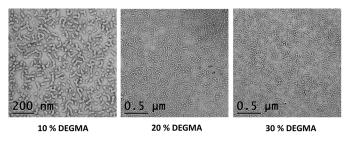
**Figure 4.** TEM images obtained for  $G_{59}$ - $(H_x$ -stat- $D_y)$  prepared with 10, 20 or 30 mol% DEGMA in the core-forming statistical block (where G, H and D denote PGMA, PHPMA and DEGMA, respectively).
