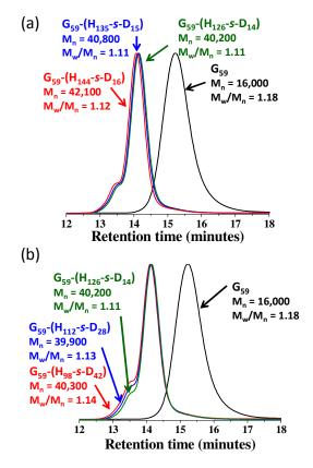
Figure 1. DMF GPC curves recorded for: (a) PGMA<sub>59</sub> and PGMA<sub>59</sub>-P(HPMA<sub>x</sub>-stat-DEGMA<sub>y</sub>) copolymers prepared with 10 mol % DEGMA in the core-forming block; (b) PGMA<sub>59</sub> and PGMA<sub>59</sub>-P(HPMA-stat-DEGMA)<sub>140</sub> copolymers comprising varying DEGMA content of the core-forming block (where G = PGMA, H = PHPMA and D = PDEGMA).
