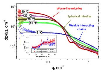
**Figure 8.** Selected SAXS patterns recorded for a 4.8% w/w aqueous dispersion of PGMA<sub>59</sub>-P(HPMA<sub>91</sub>-stat-DEGMA<sub>39</sub>) at 40°C, 25°C, 20°C, 15°C and 5°C during cooling (circles) and subsequent heating (triangles). The solid lines represent fits to the cooling data using the worm-like micelle model (at 40°C), a spherical micelle model (at 20°C) and a generalized Gaussian coil model for molecularly-dissolved copolymer chains (at 5°C). The inset shows the Porod-
