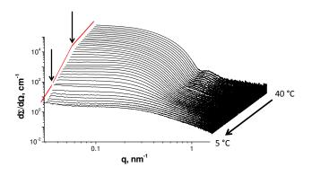
**Figure 7.** Time-resolved SAXS patterns recorded for a 4.8% w/w aqueous dispersion of PGMA<sub>59</sub>-P(HPMA<sub>91</sub>-stat-DEGMA<sub>39</sub>) during cooling from  $40^{\circ}$ C to  $5^{\circ}$ C at  $1^{\circ}$ C min<sup>-1</sup>. The solid red line indicates the reduction in SAXS intensity at low q during cooling.
