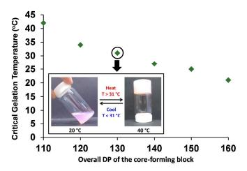
**Figure 3.** Variation of the critical gelation temperature (CGT) with overall DP of the core-forming block (x) for PGMA<sub>59</sub>-P(HPMA-stat-DEGMA)<sub>x</sub> prepared using 30 mol% DEGMA (where x = 110, 120, 130, 140, 150 or 160). Inset: digital images of PGMA<sub>59</sub>-P(HPMA<sub>91</sub>-stat-DEGMA<sub>39</sub>). A clear free-flowing liquid is obtained below the CGT of 31°C, whereas a transparent free-standing gel is formed above this CGT.
