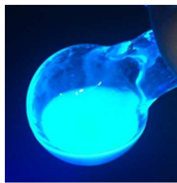
Fig. 15 Image of the reaction mixture after the “click” reaction between the alkyne functionalized PDPA and 3-azido-7-diethyl-aminocoumarin. The formation of the fluorescent linkage could be easily seen upon irradiation at 365 nm with a hand-held UV lamp.
