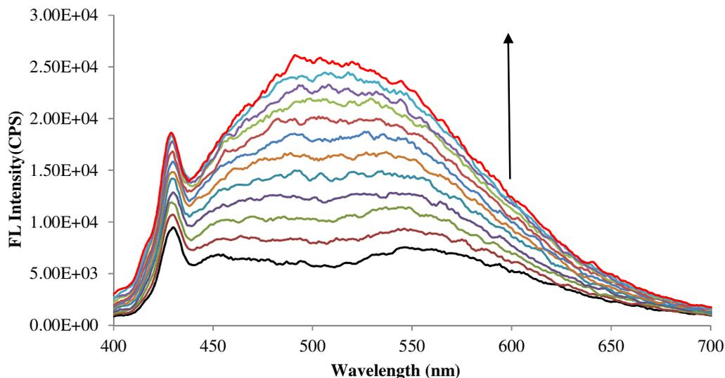
**Figure 4.** Fluorescence emission spectra of receptor **3** (10  $\mu\text{M}$ ) upon successive addition of  $\text{Co}^{2+}$  (100  $\mu\text{M}$ ) in  $\text{CH}_3\text{CN}/\text{H}_2\text{O}$  (1:1,  $v/v$ ),  $\lambda_{\text{exc}} = 405$  nm.
