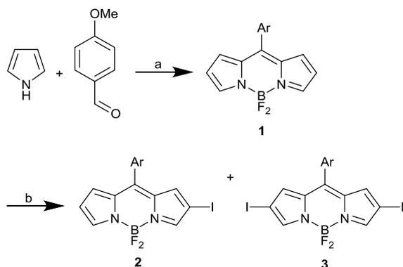
**Scheme 1.** Reagents: (a)  $\text{BF}_3 \cdot \text{OEt}_2$ , rt, 4 h (87%); DDQ,  $\text{CH}_2\text{Cl}_2$ , 0 °C, 30 min;  $\text{BF}_3 \cdot \text{OEt}_2$ ,  $i\text{-Pr}_2\text{NEt}$ , rt, 2 h (77%); (b) ICl,  $\text{CH}_2\text{Cl}_2$ -MeOH, rt, 2 h (**2**, 65%; **3**, 15%). (Ar = 4-MeOC<sub>6</sub>H<sub>4</sub>).
