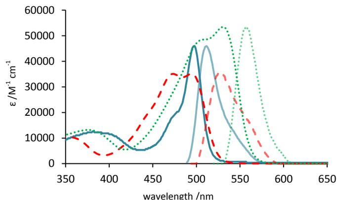
**Figure 4.** Absorption spectrum (heavy lines) in terms of the molar absorption coefficient ( $\epsilon$ ) and normalised fluorescence spectrum (feint lines) for **1** (—), **4a** (---), and **4l** (····) in THF.
