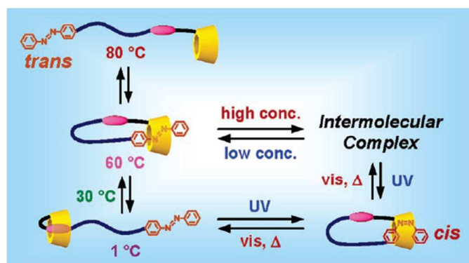
Figure 8. Proposed conformational changes of 6-Az-PEG600-HyClO- \beta -CD in aqueous solution using temperature and light. 70 Reproduced with permission from reference 70. Copyright 2007 American Chemical Society.
