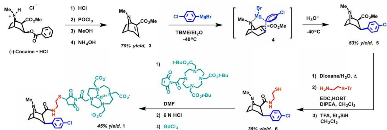
**Scheme 1** Synthesis of  $\beta$ -CCT-Derived CA, **1**. (TBME = *tert*-butyl methyl ether, EDC = 1-ethyl-3-(3-dimethylaminopropyl)carbodiimide, HOBT = hydroxybenzotriazole, DIPEA = diisopropyl ethylamine, TFA = trifluoroacetic acid.
