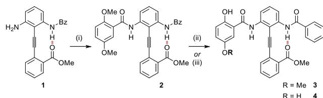
(i) 2,5-dimethoxybenzoyl chloride (2 eq.), pyridine, DMAP,  $\text{CH}_2\text{Cl}_2$ , rt, 30 min, 73%; (ii)  $\text{BBr}_3 \cdot \text{OEt}_2$  (1.5 eq.),  $-30^\circ\text{C}$ , 15 min, 94%; (iii)  $\text{BBr}_3 \cdot \text{OEt}_2$  (5 eq.), rt, 30 min, 71%. Bz = benzoyl.
