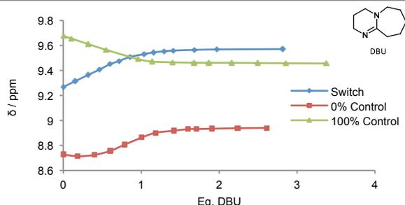
**Figure 5.**  $^1H$  NMR titration (600 MHz) of **3** (3.2 mM) with DBU (1,8-diazabicyclo[7.1.1]undec-7-ene) in  $CDCl_3$ .
