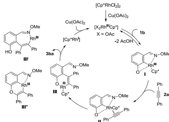
**Scheme 4** Proposed mechanism for Rh<sup>III</sup>-catalyzed benzofuran formation.
