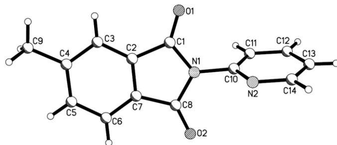
Figure 2. Molecular structure of 5-methyl-2-(pyridin-2-yl)isoindoline-1,3-dione. Displacement ellipsoids correspond to 50% probability.
