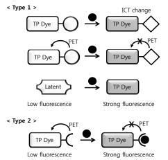
Scheme 1. Category of fluorescence probes: reaction-based (type 1) and coordination-based (type 2) probes. Black circle indicate an analyte.
