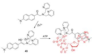
Scheme 18. Schematic illustration for the binding mode between Zn(DPA) complex **43** and ATP.
