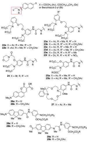
Scheme 15. Two-photon probes for  $Ca^{2+}$  (22–24),  $Mg^{2+}$  (25, 26, 28, and 29), and  $Na^{+}$  (27).
