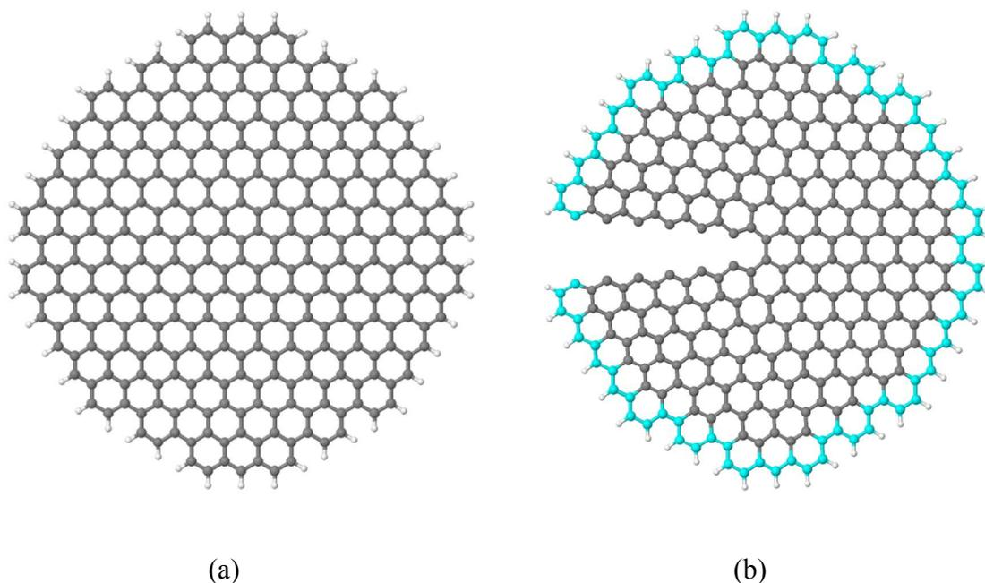
**Figure 3.** The atomistic crack tip model: (a) original configuration (b) with displacement field applied and geometry optimized. Boundary atoms (highlighted in cyan) are held fixed during the relaxation.
