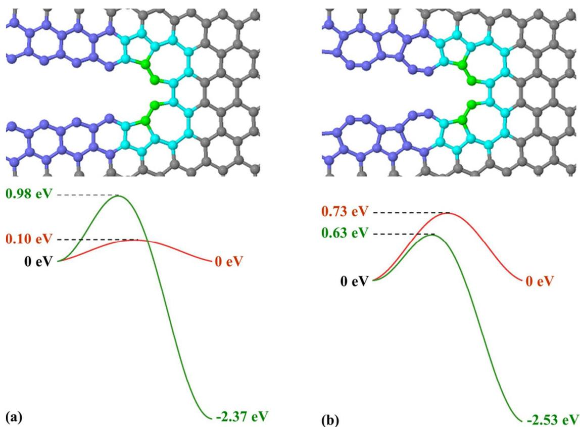
**Figure 6.** Structural and energetic comparison between first-step (a) and subsequent (b) crack tip reconstructions. The red lines are for bond breaking and the green lines are for reconstruction. Both energy reward and transition barrier show that once reconstruction is initiated, its propagation becomes much easier, suggesting the possibility of obtaining
