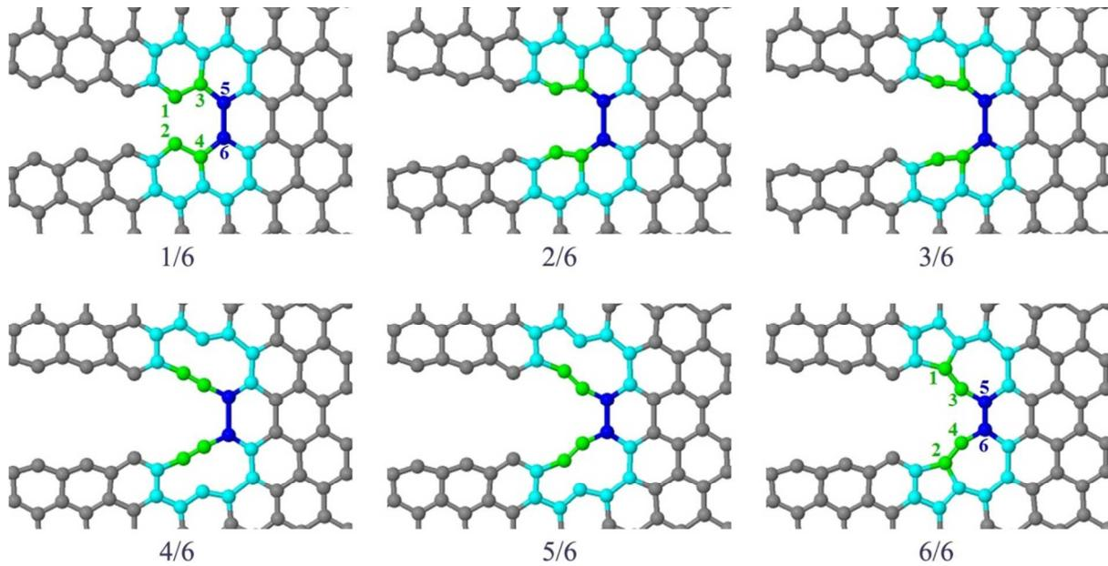
**Figure 2.** The mechanism of crack tip edge reconstruction during graphene fracture. As a result of the rotation of a pair of bonds (highlighted in green) near crack tip induced by the critical bond (highlighted in blue), the affected hexagonal cells (Step 1) gradually reconstruct into two pentagon-heptagon pairs (Steps 2-6).
