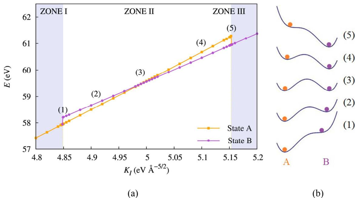
**Figure 5.** The energetics of lattice trapping effect. (a) The three zones and the butterfly pattern in Zone II (b) Total energy dependence of the model going from State A to State B, under different loads. (Inspiration of plot from SL Zhang *et al.*<sup>32</sup>)
