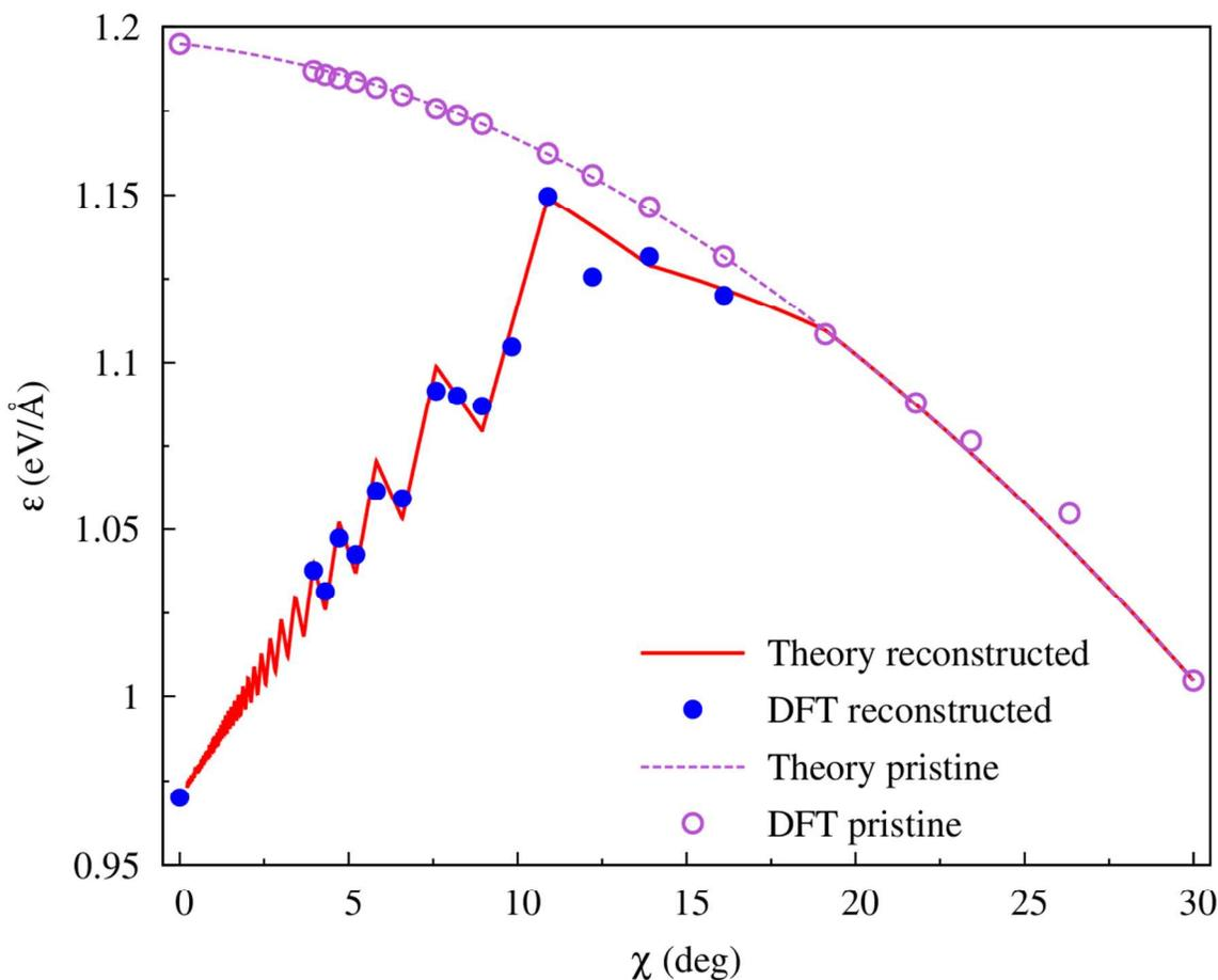
**Figure 1.** Energies per unit length of pristine and reconstructed edges: comparison between analytical formula eq 4 and DFT simulations. We can see that ZZ57 edges and AC edges are most energetically favorable among edges of all directions.
