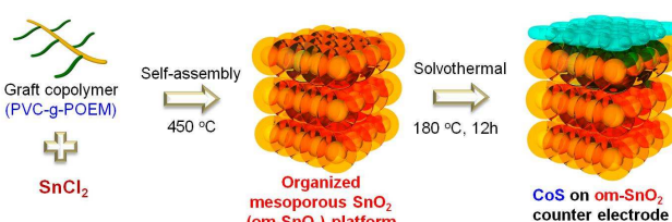
Figure 1. Schematic illustration of the preparation process of the CoS nanoparticles on om-SnO 2 platform-based counter electrode.
