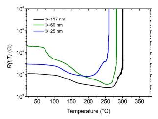
Figure 5: The impact of diameter on the response of AgNW networks to temperature when thermal ramps are used from room temperature at a rate of 2 °C per minute. The three AgNW networks have similar areal mass density of  $\approx 50 \text{ mg/m2}$ .
