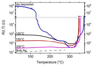
Figure 4: Temperature dependence of the electrical resistance R(t,T) of silver nanowire networks (concentration of 0.75 mg/mL) during a ramp thermal annealing of 15 °C per minute for 4 different samples: as-deposited and preannealed at 100 °C, 150 °C and 200 °C. The dashed curve is associated with the temperature-dependence of bulk silver resistivity, showing a good agreement between experimental data and phonon-induced increase of R(t,T) for the 200 °C pre-annealed specimen up to 200 °C.
