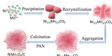
Fig. 3 Schematic diagram for the formation of \text{Ni}_{1/3}\text{Mn}_{2/3}\text{CO}_3 tremella-like structure and porous \text{NiMn}_2\text{O}_4/\text{C} nanostructures.
