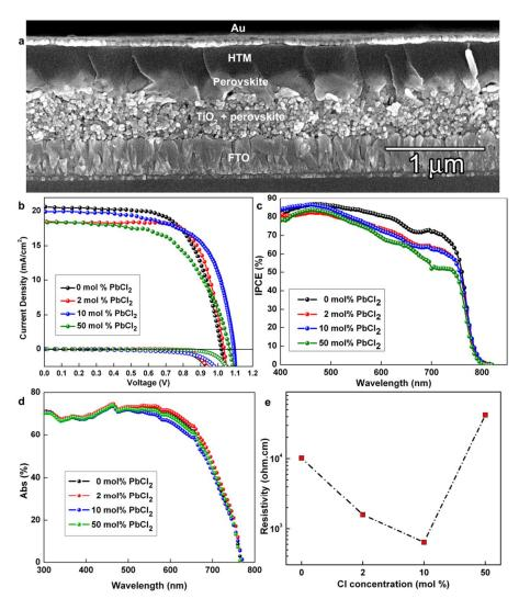
Fig3 (a) Cross-sectional FESEM image of a full device, (b) J-V and (c) IPCE of the champion cells, (d) optical absorption spectra of perovskites with different initial PbCl<sub>2</sub> concentrations on mesoporous TiO<sub>2</sub> and (e) four probe resistivity of representative perovskite films.
