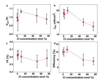
Fig.4 Statistical distribution of J-V parameters with varying Cl concentration (mol %).
