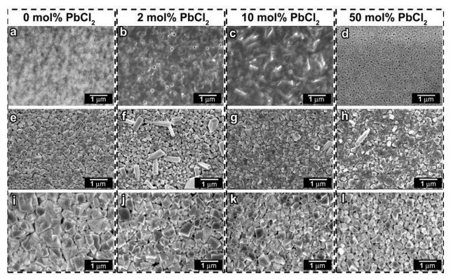
Fig.2 Top-view FESEM images illustrating surface coverage and morphological evolution with addition of Cl. (a,b,c & d) represent PbI<sub>2</sub>+ x mol % PbCl<sub>2</sub> (x being 0, 2, 10 and 50 respectively) samples, whereas (e,f,g & h) represent their corresponding morphologies after perovskite conversion when annealed at 70 °C and at 100 °C (i,j,k & l).
