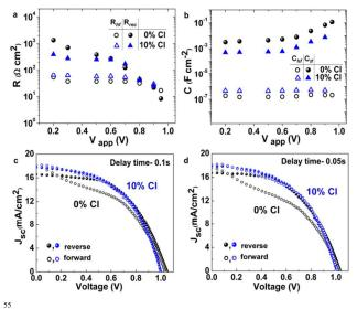
**Fig.5** (a) Resistance vs. applied voltage where the filled symbols denote  $R_{rec}$  while  $R_{HF}$  is represented by the empty symbols, (b) Capacitance vs. applied voltage plots with the filled symbols marking  $C_{LF}$  and the empty ones that of  $C_{HF}$  and (c) and (d) illustrate the hysteresis for the chlorine free and 10 mol % of PbCl<sub>2</sub> perovskite cells at different scan rates.
