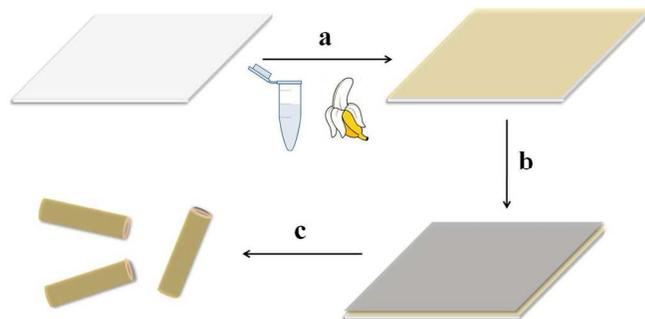
**Scheme 1.** Preparation of rolled-up tubular microengines using banana fruit cells: (a) deposition of banana fruit cells on the glass cover slip, (b) deposition of Pt layer by sputtering, (c) ultrasonication of the cells/Pt-coated cover slip.
