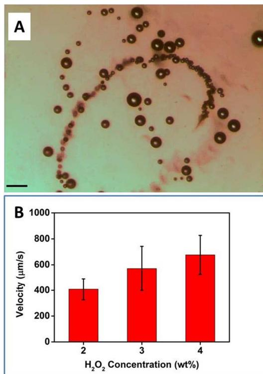
**Figure 5.** (A) Snapshot of the motion of a microtube engine in 3% H<sub>2</sub>O<sub>2</sub> and 0.5% SDS. Scale bar: 50 μm. (B) Dependence of microjets' speed on H<sub>2</sub>O<sub>2</sub> concentration in the presence of 0.5% SDS. Tracking data was obtained from 15 independent running experiments in order to obtain the average speed.
