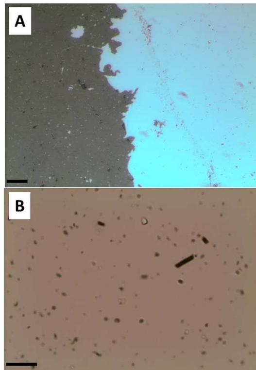
**Figure 4.** (A) Optical image of the cover slip half coated with banana fruit cells (right side) after deposition of Pt and ultrasonication in water. Platinum is still on the uncoated cover slip after ultrasonication (left side). Scale bar: 50  $\mu\text{m}$  (B) Optical image of tubular microengines fabricated using apple fruit cells. Scale bar: 20  $\mu\text{m}$ .
