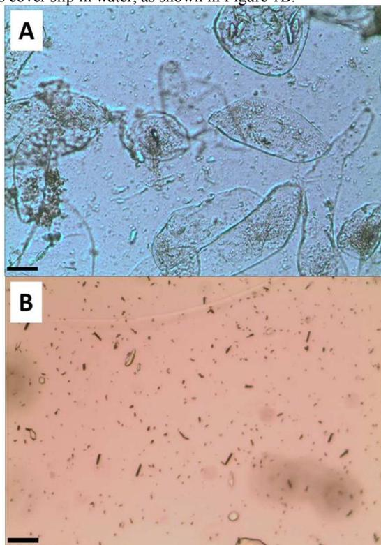
**Figure 1.** Optical images of aqueous dispersion of (A) banana fruit cells and (B) tubular microengines obtained upon ultrasonication. Scale bar: 50  $\mu\text{m}$ .
