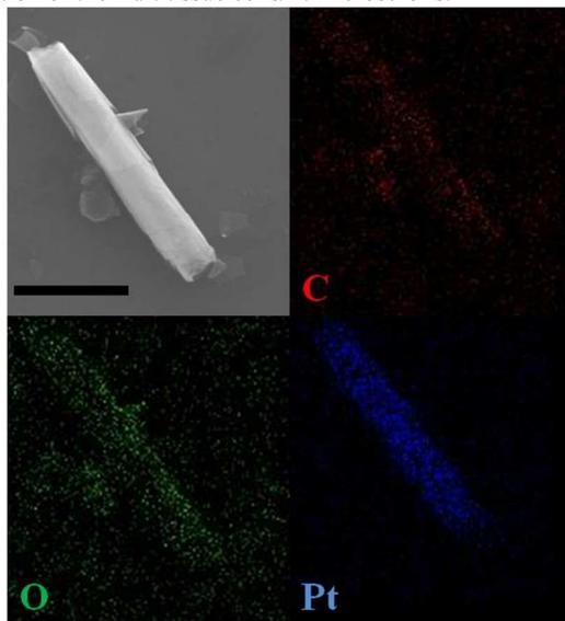
**Figure 3.** SEM/EDX elemental characterization of the tubular microengines composition. Scale bar: 10  $\mu\text{m}$ .
