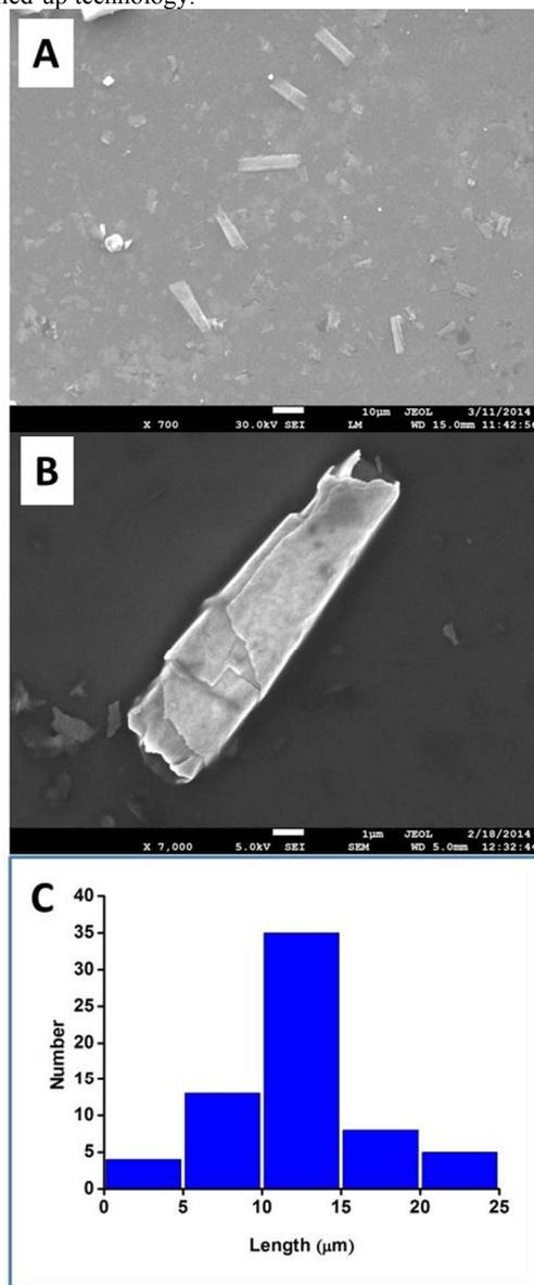
**Figure 2.** (A, B) SEM images of the fabricated tubular microengines. Scale bars are 10  $\mu\text{m}$  and 1  $\mu\text{m}$ , respectively. (C) Length distribution of the tubular microengines,  $n=65$ .
