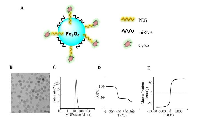
Figure.1. (A) Schematic illustration of miR16/MNPs. (B) Morphological observations of MNPs. Scale bar = 50 nm. (C) Particle size distribution of MNPs. (D) The organic content of MNPs. (E) Magnetization of MNPs.
