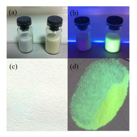
Fig. 8 (a) Daylight and (b) 365 nm UV beam photo of silica gel (left) and silica gel contain N-doped CDs (right); (c) daylight and (d) 365 nm UV beam of N-doped CDs pinned on filter paper.
