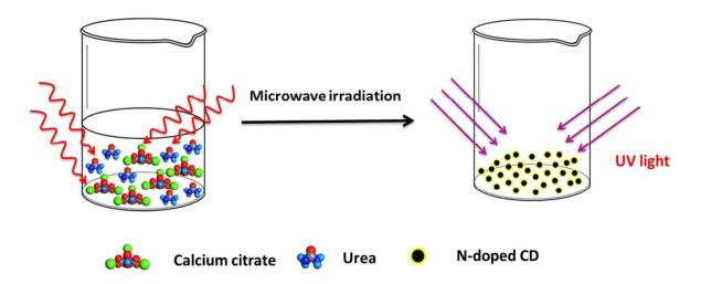
Fig. 5 Schematic diagram of the formation mechanism of N-doped CDs.
