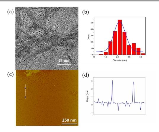
Fig. 2 (a) TEM image and (b) particle size distribution of N-doped CDs; (c) AFM image and (d) height profile of N-doped CDs.
