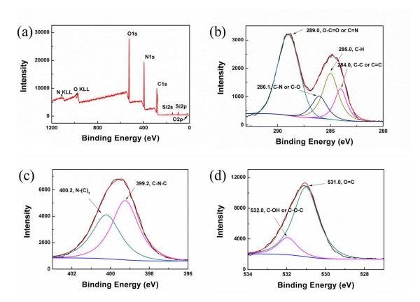
Fig. 4 XPS survey scan of N-doped CDs. (a) XPS scanning spectra show three major peaks of carbon, nitrogen and oxygen. XPS high resolution survey scan of (b) C1s, (c) N1s and (d) O1s region of N-doped CDs.
