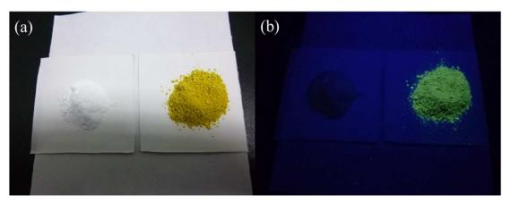
Fig. 1 The photos of calcium citrate and N-doped CDs: (a) under visible light and (b) under a 365 nm UV beam.
