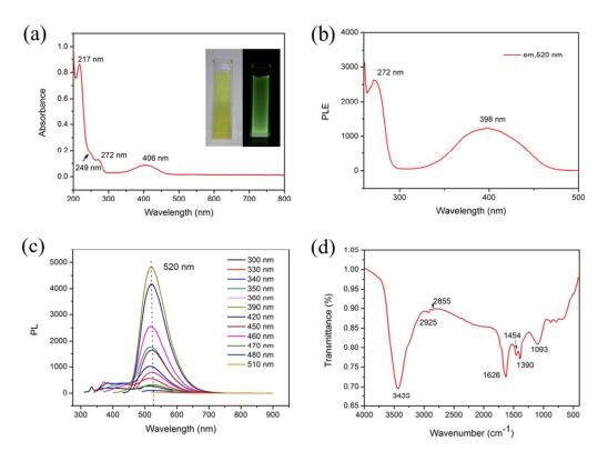
Fig. 3 (a) UV-Vis absorption spectrum of N-doped CDs, inset are photos of N-doped CDs solution under sunlight (left) and irradiated by a 365 nm UV beam (right); (b) PLE spectrum of N-doped CDs; (c) PL spectra recorded for progressively longer excitation wavelengths from 300 to 510 nm; (d) FT-IR spectrum of N-doped CDs.
