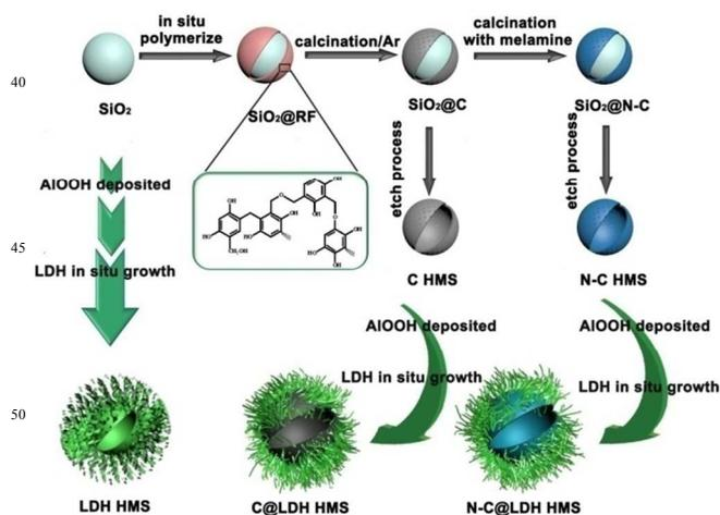
**Scheme 1** Schematic illustration for the formation process of N-C@LDH HMS, C@LDH HMS and LDH HMS.
