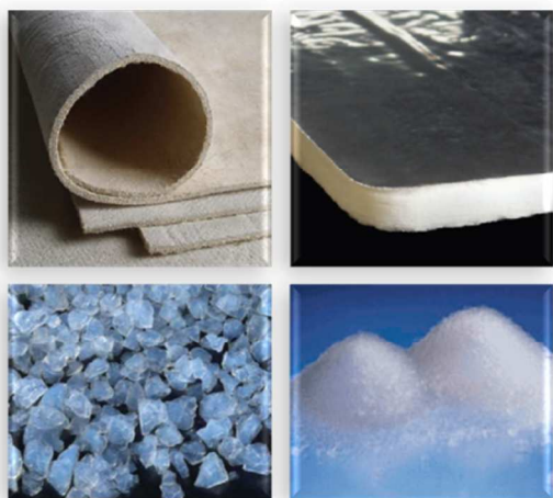
Fig. 14 Some commercial products based on hybrid O-I aerogel. Aerogel Products: Various hybrid aerogel products commercially available (top: Aspen Aerogel® flexible composite blankets / down: Nanogel™ translucent granules and fine particles - Cabot Corporation®)
