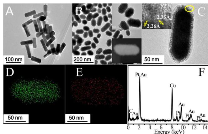
Fig. 1 Morphology and composition characterizations of Au@Pt nanostructures. (A) & (B) Low-magnification TEM images of Au NRs (A) and Au@Pt nanostructures (B). (C) High-magnification TEM image of an Au@Pt nanohybrid with crystal-lattice mapping of the area enclosed by the yellow circle shown in the inset. (D-F) Elemental mapping of Au (D) and Pt (E) in the Au@Pt nanostructure and the corresponding EDX spectrum from Au@Pt nanohybrids (F).
