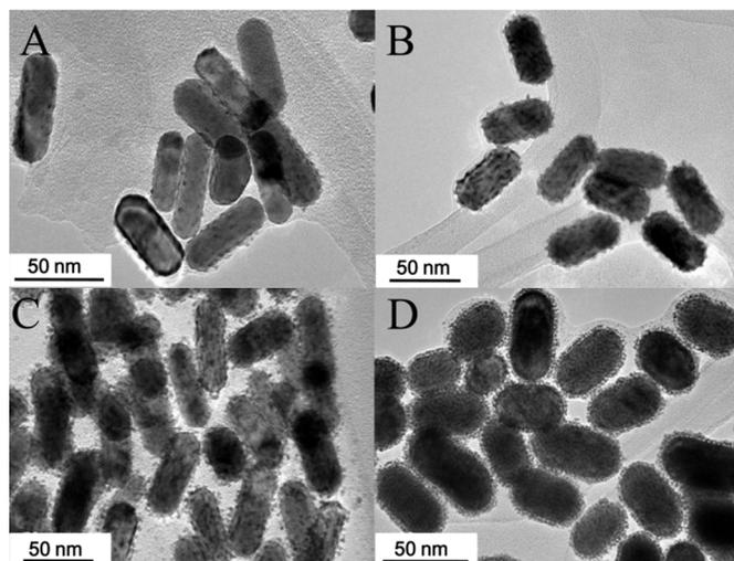
Fig. 2 (A-D) TEM images of the Au@Pt hybrid nanostructures with gradual increase in the surface coverage of Pt NPs on Au NRs. They were labelled as Au@Pt-a, Au@Pt-b, Au@Pt-c, and Au@Pt-d, respectively.
