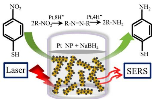
Scheme 1 Representation of the reduction of 4-NTP by NaBH<sub>4</sub> to 4-ATP, which takes place on Au@Pt superstructure surfaces. The reaction is catalyzed by the Pt NPs, while the SERS signal is brought about by local optical fields of the Au NRs.
