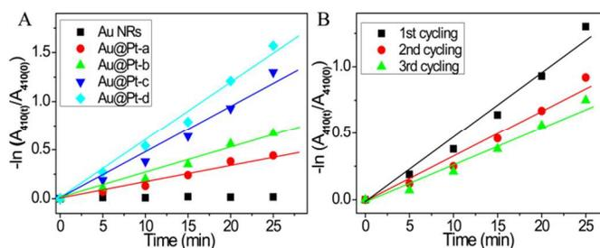
Fig. 5 (A) Plots of  $\ln(A_{410(t)}/A_{410(0)})$  as a function of reaction time for the reactions catalyzed by Au NRs, Au@Pt-a, b, c, and d nanostructures samples, respectively. (B) Three cycles of catalytic activity of the Au@Pt-c hybrids in decomposing 4-NTP. The solid lines are linear fits to the measured data points (symbols).
