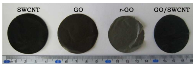
Figure 2 Digital images of as-prepared SWCNT, GO, r -GO and GO/SWCNT hybrid films
