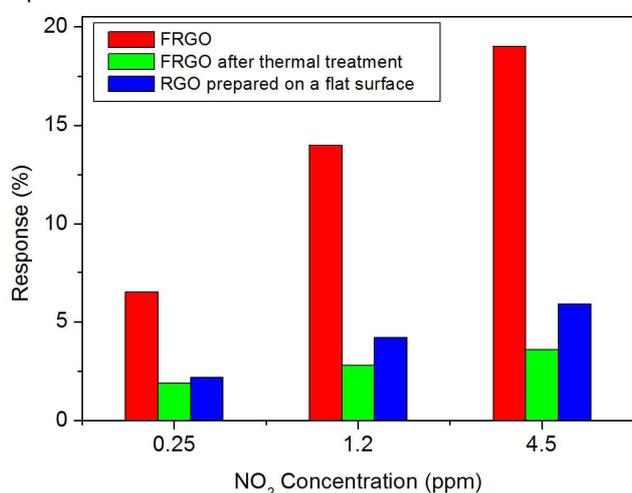
Fig. 4. Comparison of gas response depending on graphene-based gas sensor devices.
