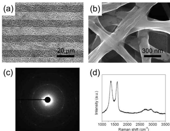
**Fig. 2** (a) SEM image of RGO nanofibers on Pt IDE for gas sensing (scale bar = 20 μm). (b) Magnification of Fig. 2(a) (scale bar = 300 nm). (c) SAED pattern of an edge of a RGO nanofiber. (d) Raman spectrum of a RGO fiber.
