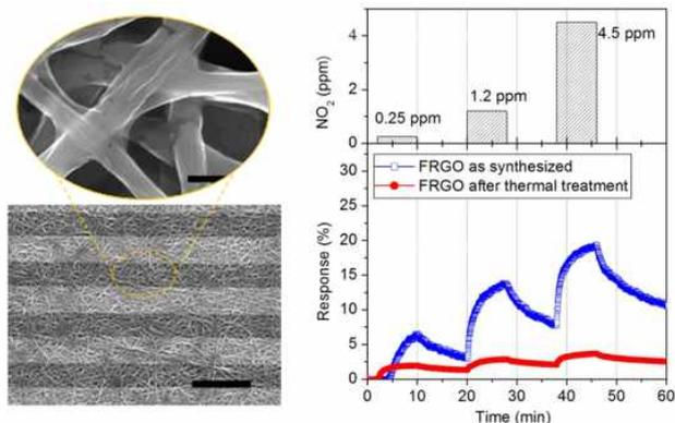
Ultra-sensitive RGO gas sensors with a facile preparation method are presented. The gas sensor composed of RGO nanofiber showed excellent sensitivity to NO<sub>2</sub> gas.
