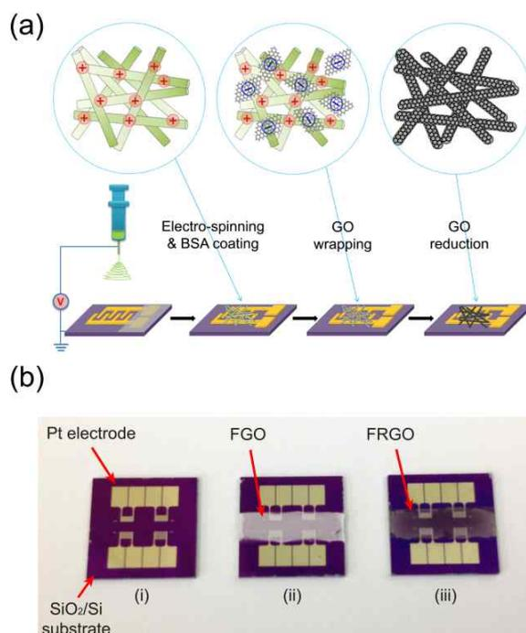
**Fig. 1** (a) Schematic illustration of the fabrication steps of FRGO gas sensors. (b) Optical images of bare device (i), GO/Nylon-6 device, FGO (ii), and gas sensing device based on reduced GO/Nylon-6, FRGO (iii).
