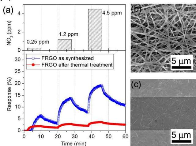
**Fig. 3** (a) Gas responses of the devices consisting of FRGO as synthesized (blue line) and FRGO after thermal treatment at 300°C (red line). SEM images of (b) FRGO as synthesized and (c) FRGO after thermal treatment at 300°C.
