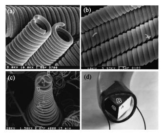
**Figure 9** Representative enlarged views of double helical (a) circular CNFs and (b) flat CNFs; (c) Enlarged view of the tip of the as-grown helical CNF (arrow indicates a Ni catalyst grain); (d) Schematic image of growth mechanism of the helical CNFs.<sup>85</sup> Reprinted with permission from Ref. 85. Copyright 1999 from American Institute of Physics.
