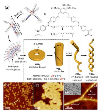
**Figure 2** (a) Schematic representation of the hierarchical selfassembly of the chiral azobenzene dimmer; (b) Atomic force microscopy height images of (b) toroidal aggregates Agg<sub>II</sub>, (c) tubular aggregates Agg<sub>II</sub> and (d) helical aggregates Agg<sub>III</sub> and Agg<sub>IV</sub>. Inserted image in (d) is the TEM image of helical aggregates Agg<sub>III</sub> and Agg<sub>IV</sub>. Reprinted with permission from Ref. 27. Copyright 2012 from American Chemical Society.
