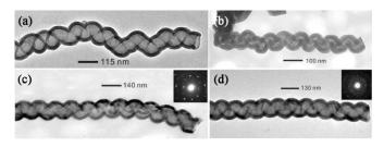
**Figure 6** TEM images of the as-fabricated helical by (a)  $Al_2O_3$ , (b)  $SiO_2$ , (c)  $TiO_2$ , and (d)  $ZnAl_2O_4$  by ALD the oxides on the surface of helical CNFs.<sup>65</sup> Reprinted with permission from Ref. 65. Copyright 2010 from Wiley-VCH.
