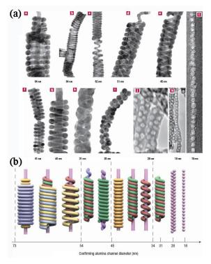
**Figure 7** (a) Representative TEM images of mesostructures formed inside PAA nanochannels with differing confinement dimensions; (b) Summary of the experimentally observed confined mesostructural evolution with varying alumina nanochannel diameters.<sup>72</sup> Reprinted with permission from Ref. 72. Copyright 2004 from Nature Publishing Group.
