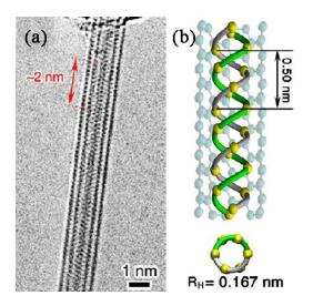
**Figure 8** (a) High-resolution TEM image revealing the Se doublehelix structure with a pitch length of  $\sim$ 2 nm inside a DWCNT; (b) The optimized structure of a free-standing double-helix structure of selenium inside the (5,5) CNT.<sup>74</sup> Reprinted with permission from Ref. 74. Copyright 2013 from American Chemical Society.
