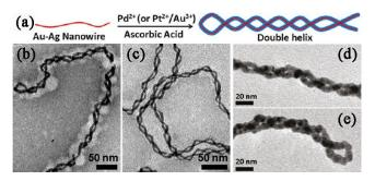
**Figure 12** (a) Schematics illustrating the formation of double helix by growing a metal layer on Au-Ag alloy nanowire; TEM images of the (b, c) (Au-Ag)@Pd and (d, e) (Au-Ag)@Au double helices.<sup>13</sup> Reprinted with permission from Ref. 13. Copyright 2011 from American Chemical Society.
