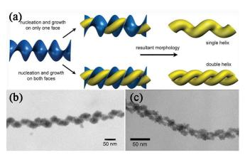
**Figure 5** (a) Schematic representation of templating pathways. Nucleation and growth on one side of the twisted ribbons (blue) leads to single helices of CdS (yellow), while nucleation and growth on both sides of the ribbon leads to double helices; TEM images of a CdS (b) single helix and (c) double helix.<sup>60</sup> Reprinted with permission from Ref. 60. Copyright 2005 from Wiley-VCH.
