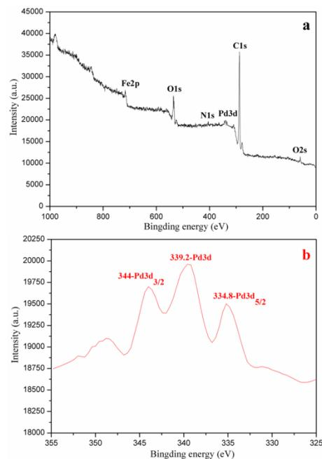
Fig. 8 XPS spectra of Fe<sub>3</sub>O<sub>4</sub>/DA-Pd<sup>II</sup> after 5 cycles of the reaction
