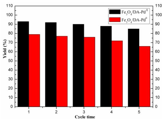
Fig. 9 Recyclability of Fe<sub>3</sub>O<sub>4</sub>/DA-Pd<sup>II</sup> and Fe<sub>3</sub>O<sub>4</sub>/DA-Pd<sup>0</sup> for the Suzuki carbonylative cross-coupling reaction of iodobenzene with phenylboronic acid
