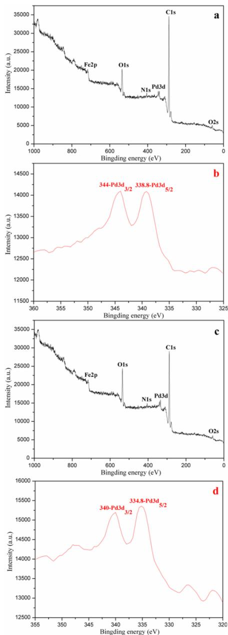
Fig. 5 XPS spectra of (a, b)  $\text{Fe}_3\text{O}_4/\text{DA-Pd}^{\text{II}}$  and (c, d)  $\text{Fe}_3\text{O}_4/\text{DA-Pd}^0$
