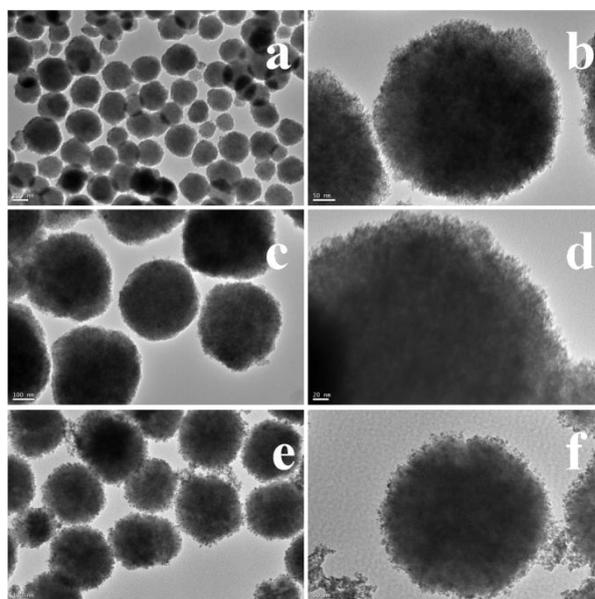
Fig. 1 TEM images of (a, b) Fe<sub>3</sub>O<sub>4</sub>/DA, (c, d) Fe<sub>3</sub>O<sub>4</sub>/DA-Pd<sup>II</sup> and (e, f) Fe<sub>3</sub>O<sub>4</sub>/DA-Pd<sup>0</sup>
