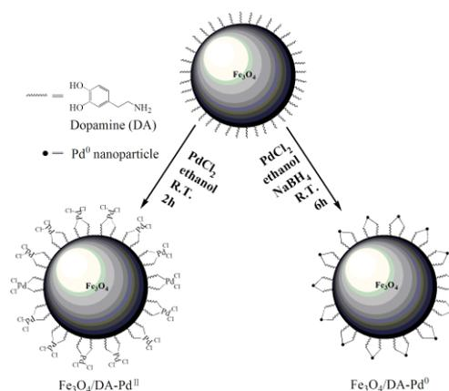
Scheme 1 Preparation of Fe<sub>3</sub>O<sub>4</sub>/DA-Pd<sup>II</sup> and Fe<sub>3</sub>O<sub>4</sub>/DA-Pd<sup>0</sup> catalysts
