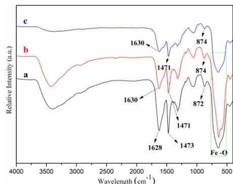
Fig. 4 FT-IR spectra of (a)  $\text{Fe}_3\text{O}_4/\text{DA}$ , (b)  $\text{Fe}_3\text{O}_4/\text{DA-Pd}^{\text{II}}$  and (c)  $\text{Fe}_3\text{O}_4/\text{DA-Pd}^0$
