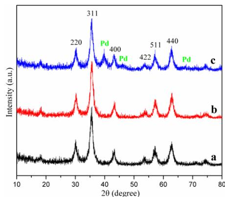
Fig. 3 XRD patterns of (a)  $\text{Fe}_3\text{O}_4/\text{DA}$ , (b)  $\text{Fe}_3\text{O}_4/\text{DA-Pd}^{\text{II}}$  and (c)  $\text{Fe}_3\text{O}_4/\text{DA-Pd}^0$
