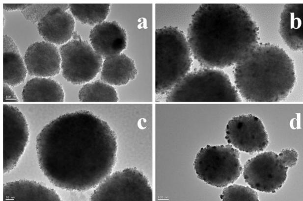
Fig. 7 TEM images of (a) Fe<sub>3</sub>O<sub>4</sub>/DA-Pd<sup>II</sup> and (b) Fe<sub>3</sub>O<sub>4</sub>/DA-Pd<sup>0</sup> after the first cycle of Suzuki carbonylative cross-coupling reaction, (c) Fe<sub>3</sub>O<sub>4</sub>/DA-Pd<sup>II</sup> and (d) Fe<sub>3</sub>O<sub>4</sub>/DA-Pd<sup>0</sup> after 5 cycles of the reaction
