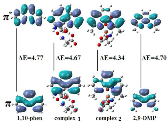
Fig. 2 Energy gaps between  $\pi$ - $\pi^*$  of the coordinated and free phenanthroline.
