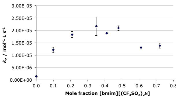
**Fig. 2** The bimolecular rate constant ( $k_2$ ) for the ethanalysis of diethyl chlorophosphate at different mole fractions of [bmim][(CF<sub>3</sub>SO<sub>2</sub>)<sub>2</sub>N] in acetonitrile at 298.2 K. Uncertainties are the standard error of the mean derived from at least three replicate measurements at each mole fraction.
