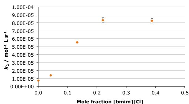
**Fig. 4** The bimolecular rate constant ( $k_2$ ) for the ethanolysis of diethyl chlorophosphate at different mole fractions of [bmim][Cl] in ethanol-*d*<sub>6</sub> at 298.2 K. Uncertainties are the standard error of the mean derived from at least three replicate measurements at each mole fraction.
