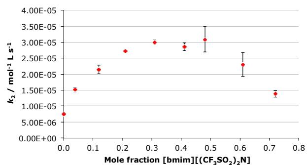
**Fig. 1** The bimolecular rate constant ( $k_2$ ) for the ethanolysis of diethyl chlorophosphate at different mole fractions of [bmim][( $CF_3SO_2)_2N$ ] in ethanol- $d_6$  at 298.2 K. Uncertainties are the standard error of the mean derived from at least three replicate measurements at each mole fraction.
