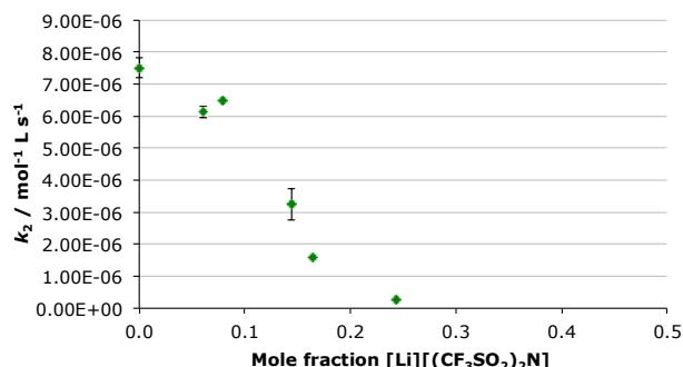
**Fig. 3** The bimolecular rate constant ( $k_2$ ) for the ethanolysis of diethyl chlorophosphate at different mole fractions of lithium bis(trifluoromethylsulfonyl)imide in ethanol-*d*<sub>6</sub> at 298.2 K. Uncertainties are the standard error of the mean derived from at least three replicate measurements at each mole fraction.
