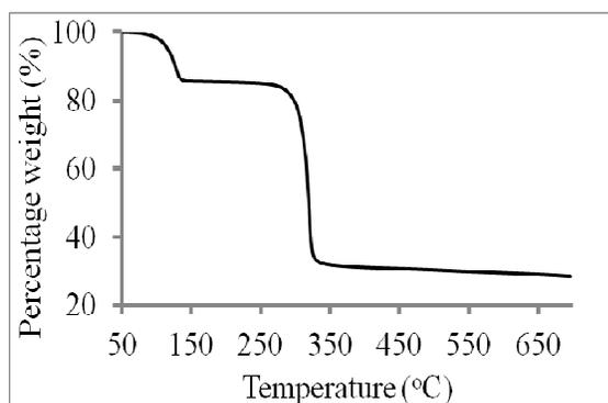
**Fig. 2** Thermogravimetric analysis (TGA) plot of the pyridine adduct  $[\text{Cd}(\text{S}_2\text{C}(\text{NC}_5\text{H}_{10}))_2(\text{NC}_5\text{H}_5)]$  at a heating rate of  $10\text{ }^\circ\text{C min}^{-1}$  under a nitrogen atmosphere.
