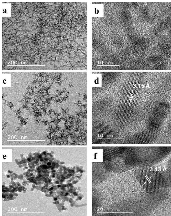
**Fig. 4** TEM and HRTEM images of HDA capped CdS nanoparticles synthesized by thermolysis of  $[\text{Cd}(\text{S}_2\text{C}(\text{NC}_5\text{H}_{10}))_2(\text{NC}_5\text{H}_5)]$  at temperatures of (a-b) 190 °C, (c-d) 230 °C and (e-f) 270 °C.
