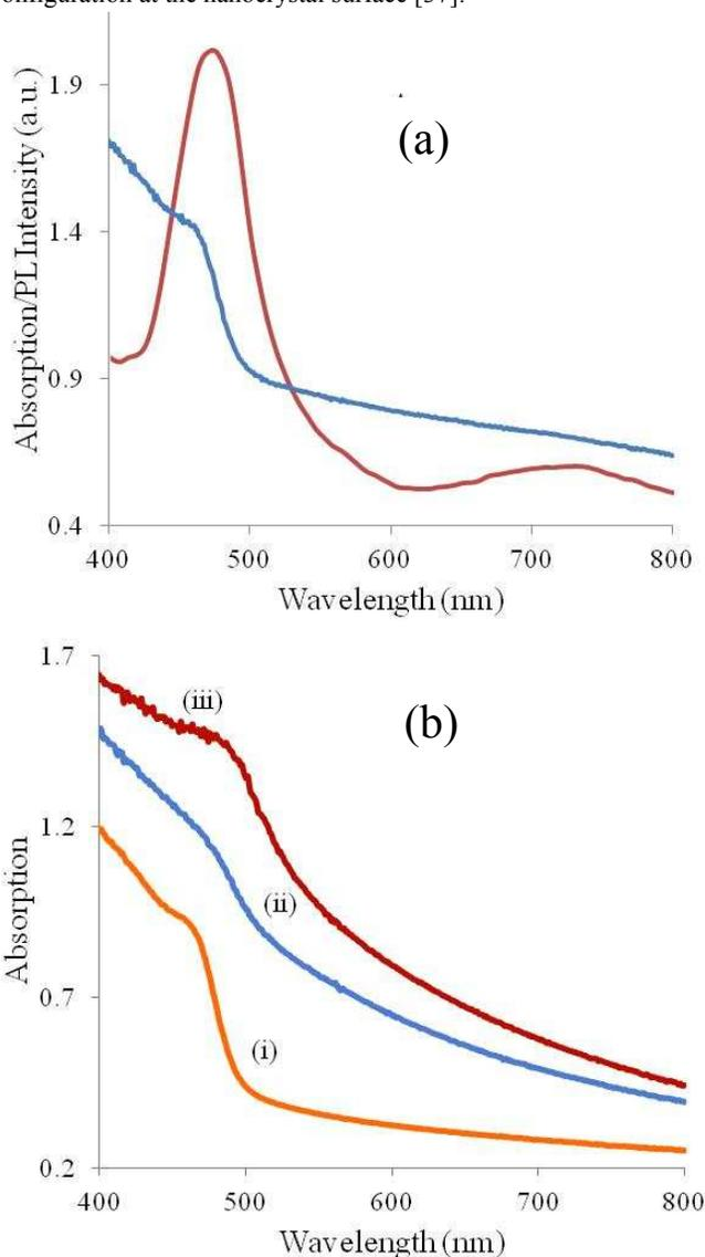
**Fig. 3** (a) UV-vis absorption (blue) and PL (red) spectra of HDA capped CdS nanoparticles at 190 °C and (b) combined UV-vis absorption spectra for CdS nanoparticles synthesized at (i) 190 °C, (ii) 230 °C and (iii) 270 °C reaction temperatures. PL spectra are corrected for instrument response.
