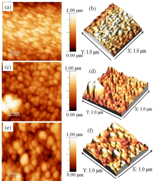
**Fig. 8** 2-D and 3-D AFM images of CdS thin films deposited by AACVD at (a and b) 350 °C, (c and d) 400 °C and (e and f) 450 °C.
