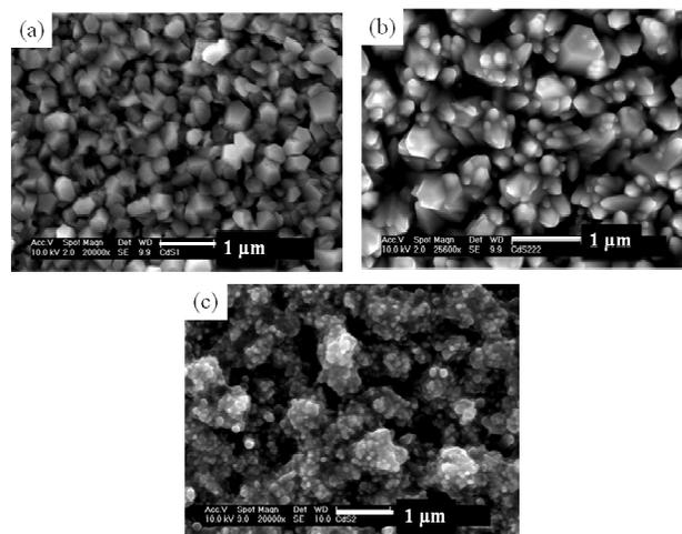
**Fig. 7** SEM images of CdS thin films deposited at (a) 350 °C, Magn. 20000X; (b) 400 °C, Magn. 2560X and (c) 450 °C, Magn. 20000X.
