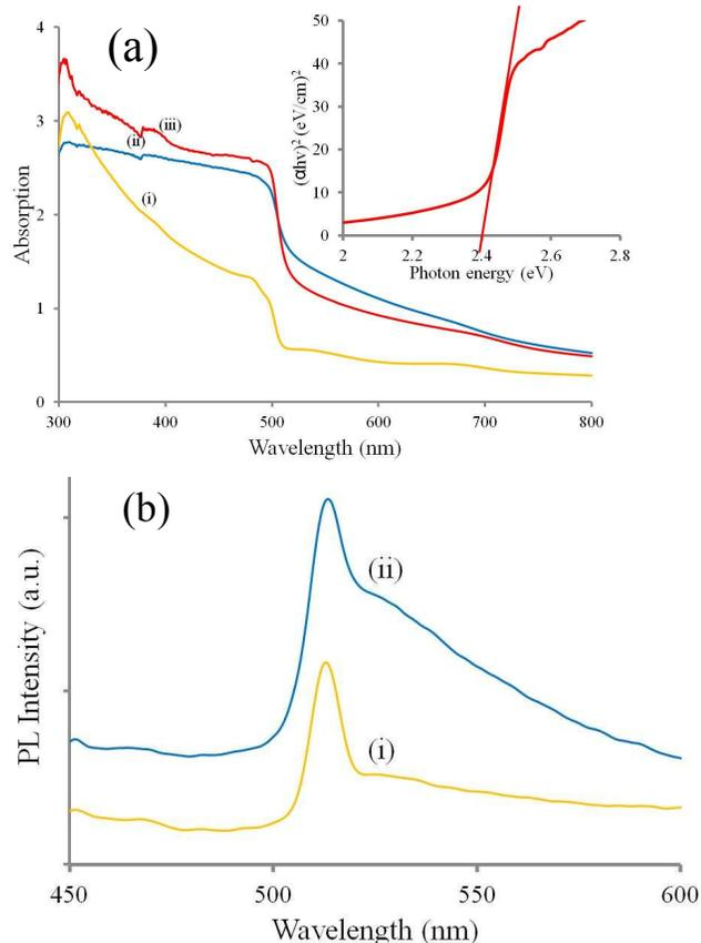
**Fig. 6(a)** UV-vis absorption of CdS thin films deposited by AACVD at (i) 350 °C, (ii) 400 °C and (iii) 450 °C. Inset: Tauc plot showing the estimated optical band gap ( $2.4 \pm 0.2$  eV). (b). Photoluminescence emission spectra of CdS thin films at (i) 350 °C and (ii) 400 °C ( $\lambda_{\text{exc}} = 350$  nm). PL spectra were corrected for instrument response.
