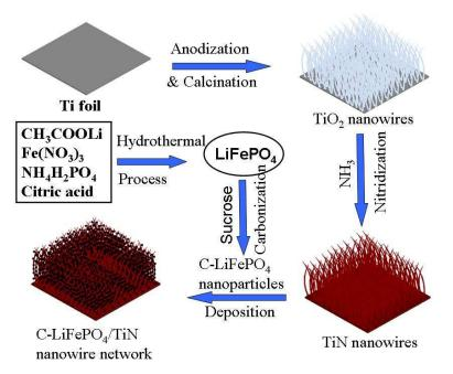
The carbon-coated lithium iron phosphate supporting on titanium nitride nanowire network was designed as the electrode material of lithium-ion supercapacitor.
