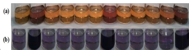
Fig. 2 Colour changes seen for receptors (a) 1 and (b) L ( 2 \times 10^{-5} mol L -1 in DMSO) after addition of 5 equiv. of various anions. From left to right: none, F - , Cl - , Br - , I - , ClO 4 - , AcO - , NO 3 - , HSO 4 - , N 3 - , NO 2 - and H 2 PO 4 - (TBA + salts).
