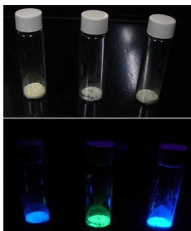
Fig 6. Picture of the compound **15** (left), **16** (right) and **17** (middle) in the solid state under irradiation of normal light (above) and UV 365nm (below).
