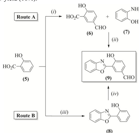
Scheme 2 Reaction pathways for obtention of formyl functionalized HBO (**9**). Conditions: (i) Hexamethylenetetramine (HMTA), acetic acid (AcOH), reflux, 8h; (ii) and (iii) **7**, polyphosphoric acid (PPA), 170°C, 5h, (iv) HMTA, PPA, 100°C, 4h.
