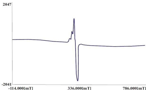
Fig. 3. EPR spectrum of the Cu(II) polymer conjugates at LNT.
