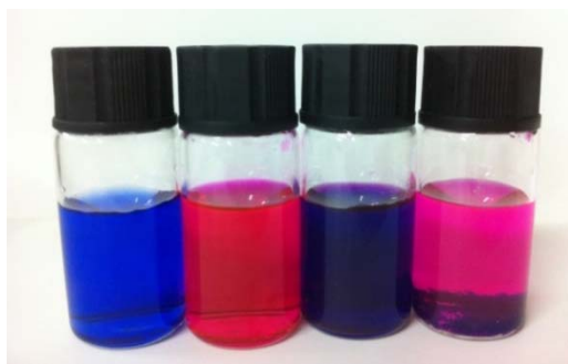
Fig. 6 Photographs showing the coloured solutions. From left to right: MB, RB, mixture of MB and RB and after addition of modified nanotubes (note the solid at the bottom of this vial which shows the blue colour of MB).
