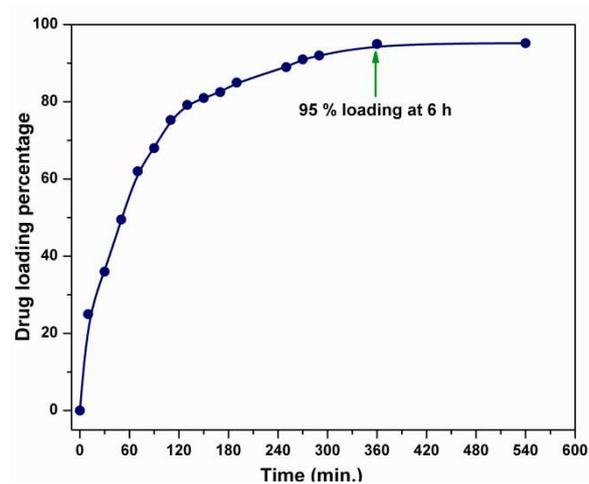
Fig. 4 Determination of drug loading efficiency of M-POSS using the model drug, Ibuprofen.
