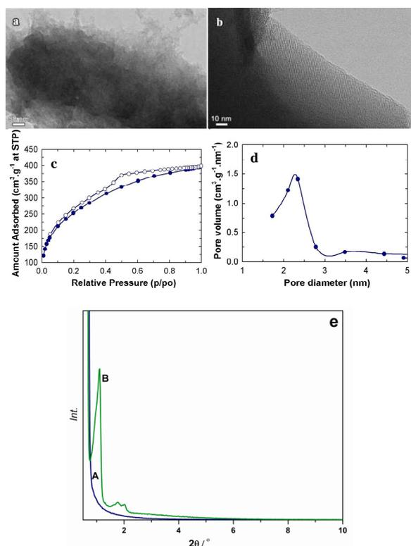
**Fig. 1** Transmission electron micrographs of as-synthesized (a) & solvent extracted (b) M-POSS, nitrogen physisorption (c) & BJH isotherms (d) of solvent extracted M-POSS and powder XRD patterns of as-synthesized (A) & solvent extracted (B) M-POSS.
