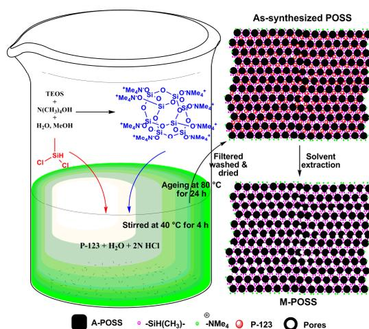
Fig. 5 Schematic representation depicting the synthesis of M-POSS.
