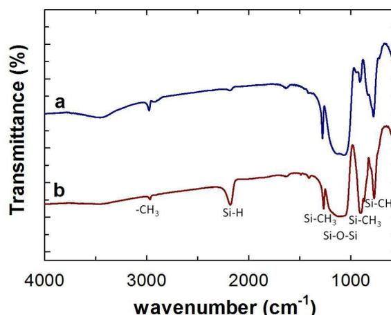
**Fig. 2** FT-IR spectra of as-synthesized (a) and solvent extracted (b) M-POSS.
