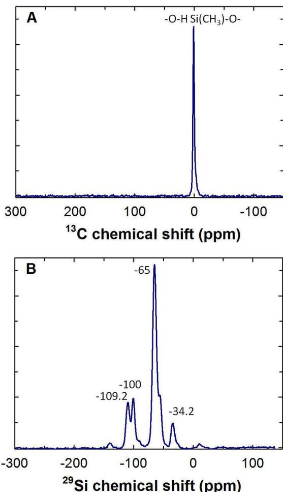
Fig. 3 CP MAS  $^{13}\text{C}$  and  $^{29}\text{Si}$ -NMR of solvent extracted M-POSS.
