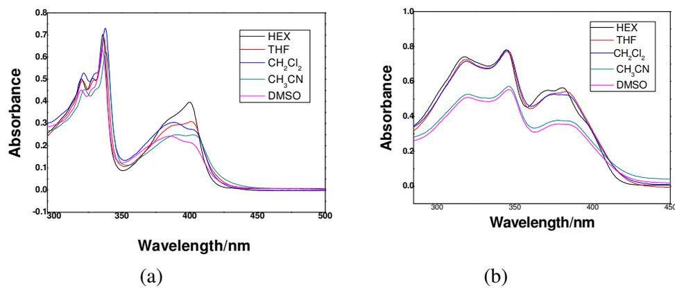
(a) the UV-vis absorption spectra of **DDBICZ** in several solvents.
