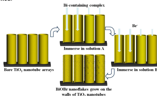
Fig.4 Schematic illustration of possible formation mechanism of BiOBr/TNTAs heterojunction
