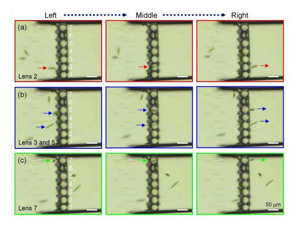
Figure 4. Center-pass function of the optofluidic device to control the cell position. (a) Microscopic images of a cell passing above lens 2. The cell is initially located at the left side of the device in the microchannel. Then it passes through the aperture in the confining wall above the center part of the lens. Finally it reaches the right side of the device. (b) and (c) Three cells pass above the centers of microlenses 3, 5, and 7 from left to right.
