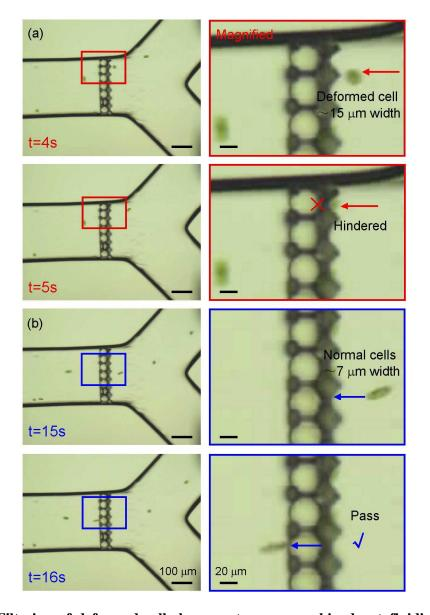
Figure 6. Filtering of deformed cells by a center-pass combined optofluidic MLA. (a) Some cells have a round shape due to biological deformation. The diameter of such cells can be as large as 15  $\mu$ m. They are hindered from passing by the 9- $\mu$ m apertures in the confining wall. (b) Normal cells with 6–8  $\mu$ m width can freely pass the apertures in the wall. Also see Supporting Video 2.
