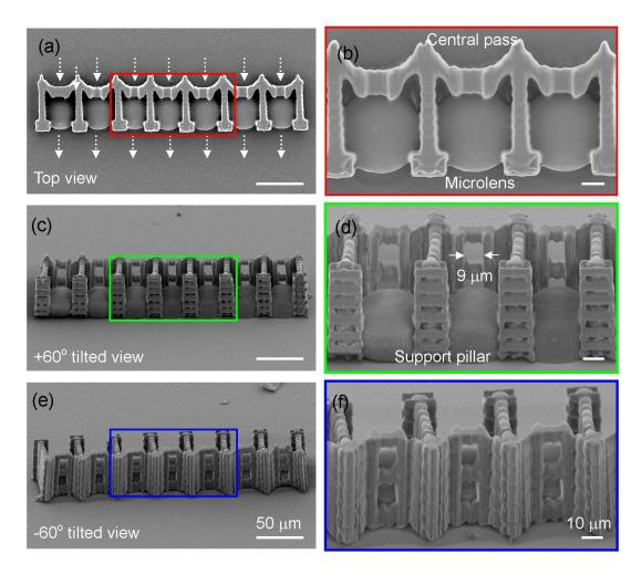
Figure 2. TPP fabrication of a center-pass combined MLA on a flat glass surface. (a)
