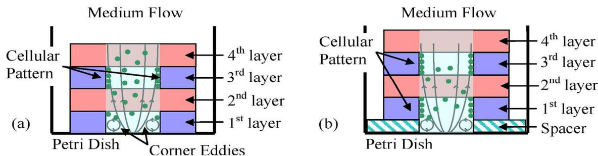
Fig. 6 Medium flow within the structure: (a) original; (b) with the spacer
