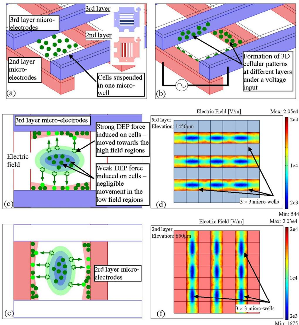
**Fig. 2** DEP cell manipulation via the multi-layer scaffold: (a) Cells in one micro-well; (b) Formation of 3D cellular pattern; (c) Cell manipulation at the 3rd layer due to the electric field; (d) electric field simulation of the 3rd layer at 10V voltage input; (e) Cell manipulation at the 2nd layer due to the electric field; (f) electric field simulation of the 2nd layer at 10V voltage input
