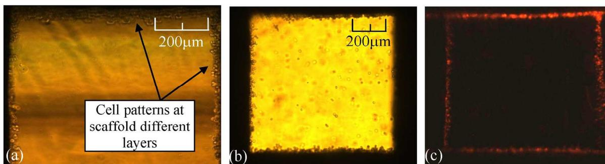
Fig. 7 3D pattern constructed from the structure with a spacer: (a) brightfield image (10×); (b) brightfield image (4×); (c) fluorescent image (4×)
