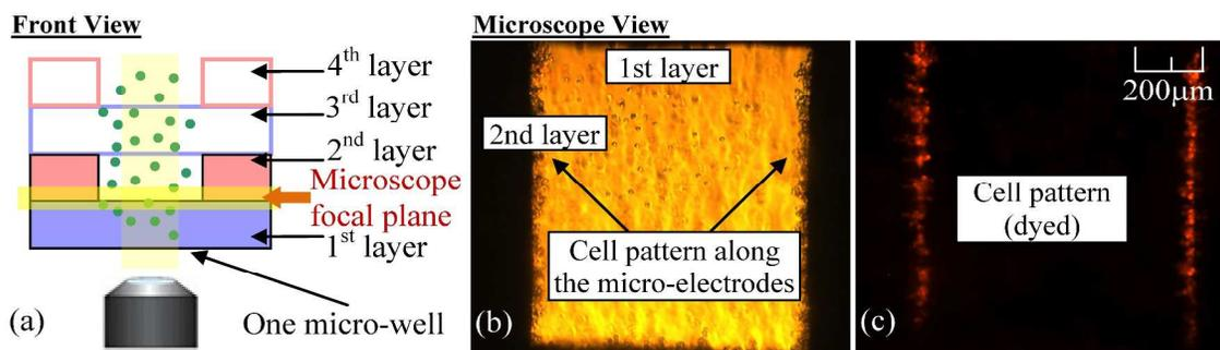
**Fig. 5** 3D pattern constructed from 3T3 cells: (a) schematic diagram; (b) brightfield image; (c) fluorescent image
