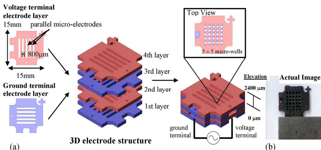
Fig. 1 (a) Schematic and (b) Photograph of the multi-layer scaffold structure for 3D cell manipulation
