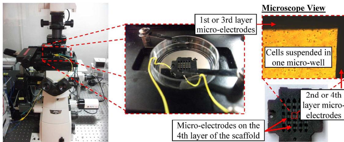
**Fig. 3** Multi-layer structure on the Eclipse Ti inverted microscope by Nikon
