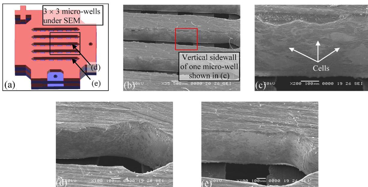
**Fig. 11** (a) 3D view of the scaffold; (b) SEM image of the micro-wells after 7 days of culture; (c) 3T3 cells on the vertical sidewall of one micro-well; (d) Micro-well with higher cell density; (e) Outermost micro-well with lower cell density
