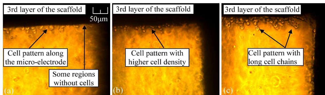
**Fig. 4** Formation of the cellular pattern at the 3rd layer under: (a) 5V; (b) 10V; and (c) 20V voltage input
