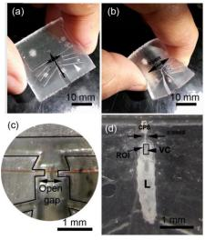
Fig. 6: Steps to load the larva using the FlexiChip. The chip is bent (b) so that the clip (c) opens. Then, the animal is inserted into the gap and the chip is released and sealed by a coverslip (d). Time-lapsed fluorescent imaging was then conducted on the CNS located inside 30 the Region of Interest (ROI)31
