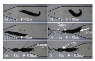
Fig. 5: Steps to load the larva using the pneumatic chip. (a-d) larva swam freely into the trap, (e-f) larva was pneumatically moved into the trap and immobilized. Time-lapsed fluorescent imaging was then 10 conducted on the CNS located inside the Region of Interest (ROI). Scale bar=400 µm for all figures is shown in Fig. 5e.
