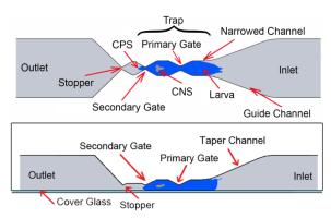
Fig. 2: Schematic design of the pneumatic chip (not to scale) topview (top image) and side view (bottom). The inlet channel was 25 mm long, 3 mm wide and 2 mm deep with an inlet port for animal 80 loading located at its end. The outlet channel was 8 mm long, 3 mm wide 2 mm deep for ejection of tested animals.
