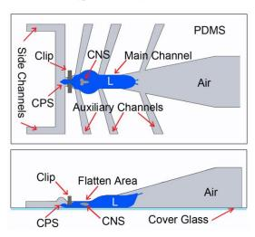
15 Fig. 3: Schematic design of the FlexiChip (not to scale) – topview (top image) and side view (bottom)
