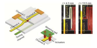
A versatile, powerless, valving and automation toolkit for paper microfluidic devices that uses absorbent expanding elements as actuators is presented.
